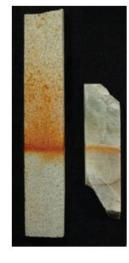
Figure 4. Secondary mineralization on sandstone and albite coupons. Note higher staining at the scCO<sub>2</sub>/water interface.
