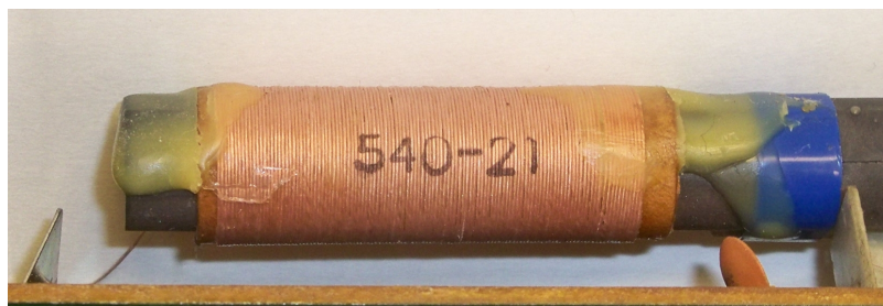
Figure 9. Ferrite rod antenna.
