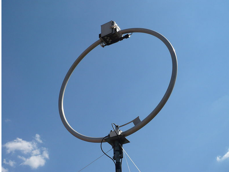
Figure 8. A resonant-loop antenna tuned for short-wave reception (Source: Wikipedia Commons).
