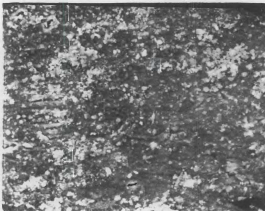
FIGURE 103. SEM View of Fission Products on Inner Cladding Surface from Rod R1 (1250X)
