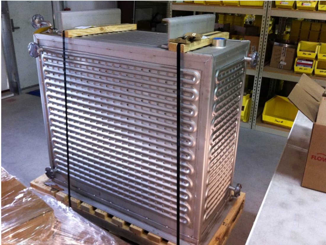
Figure 4 – 100kWh t prototype enclosure made of Flat-Panel Open Tank Heat Exchanger panels.
