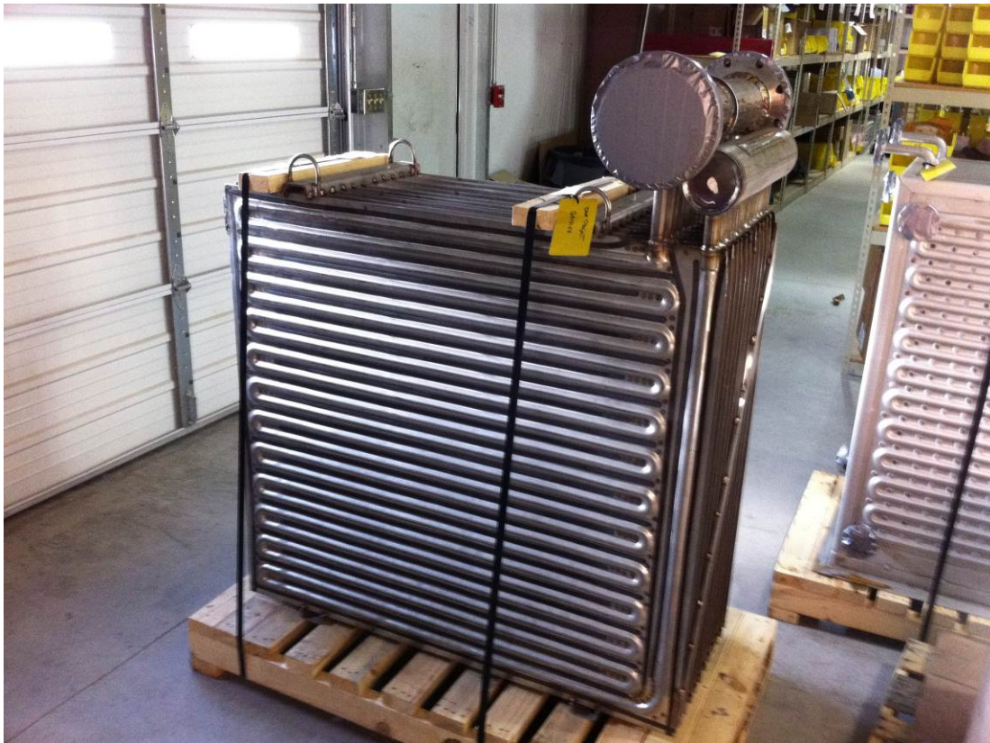
Figure 3 – 100kWh t prototype HEX bank made of 12 Flat-Panel Open Tank Heat Exchanger.
