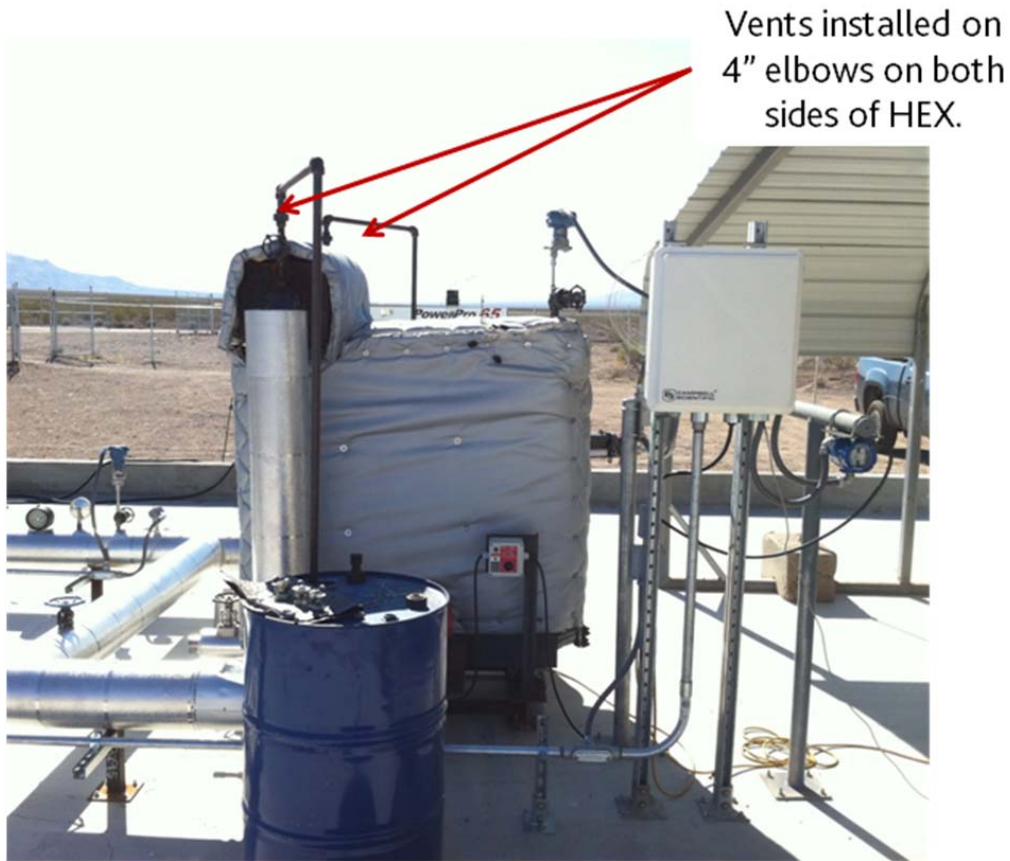
Figure 26 – Prototype heat exchanger after test loop modifications.
