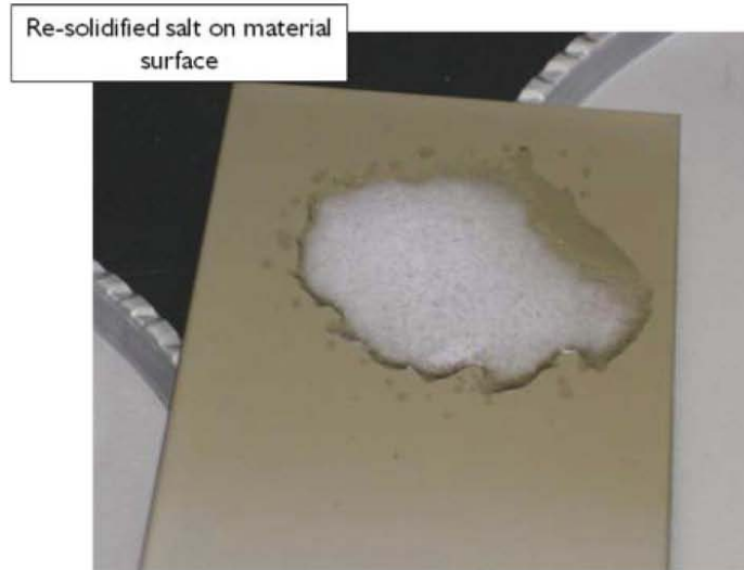
Figure 5 – Coupon after removal from hot plate and PCM solidification.
