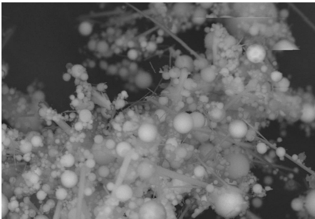
Figure 20. Fly ash after 24 hours of hydration at natural pH showing ettringite formation (2500x).
