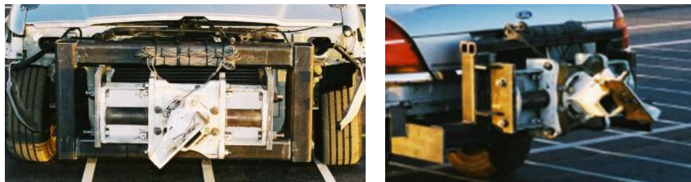
Figure 3.2: CRIS cradle mounted on the Crown Victoria's (a) front (b) back.
