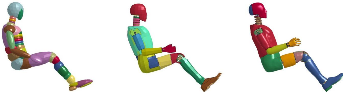
Figure 7.5: Neutral position of the MADYMO dummy (left), the LSTC Fast dummy (middle) and the NCAC detailed dummy (right).
