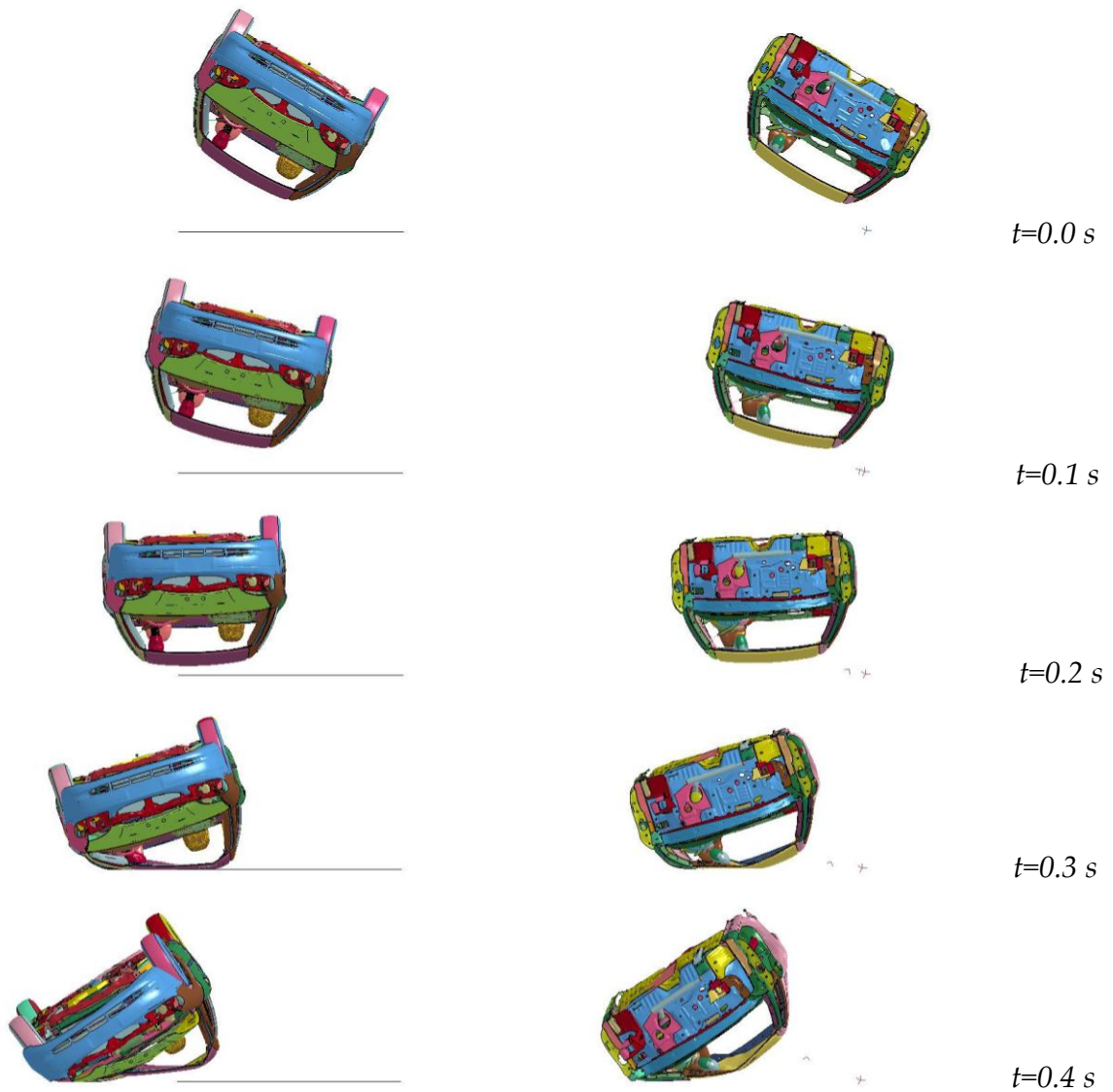
Figure 4.1: Comparison of vehicle kinematics and deformations in (left) TRACC simulation with NCAC dummy (right) NHTSA simulation with MADYMO dummy.
