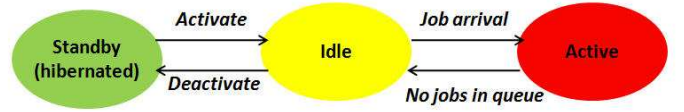
Fig. 1. Power state transition diagram of a node in the cluster (we omit Power-off state.)
