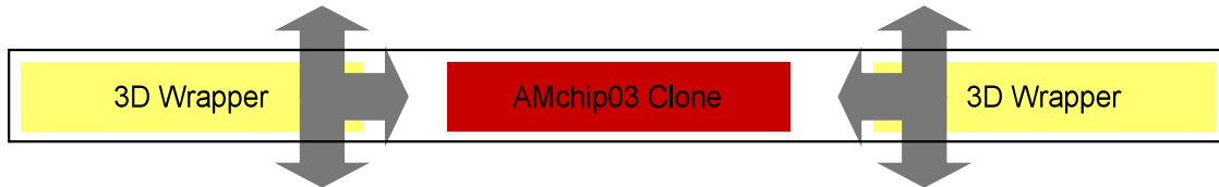
Figure 4. 3D integration of AMchip03 wrapped with IO interface.
