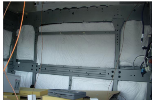
Figure 11. Insulation Package I
