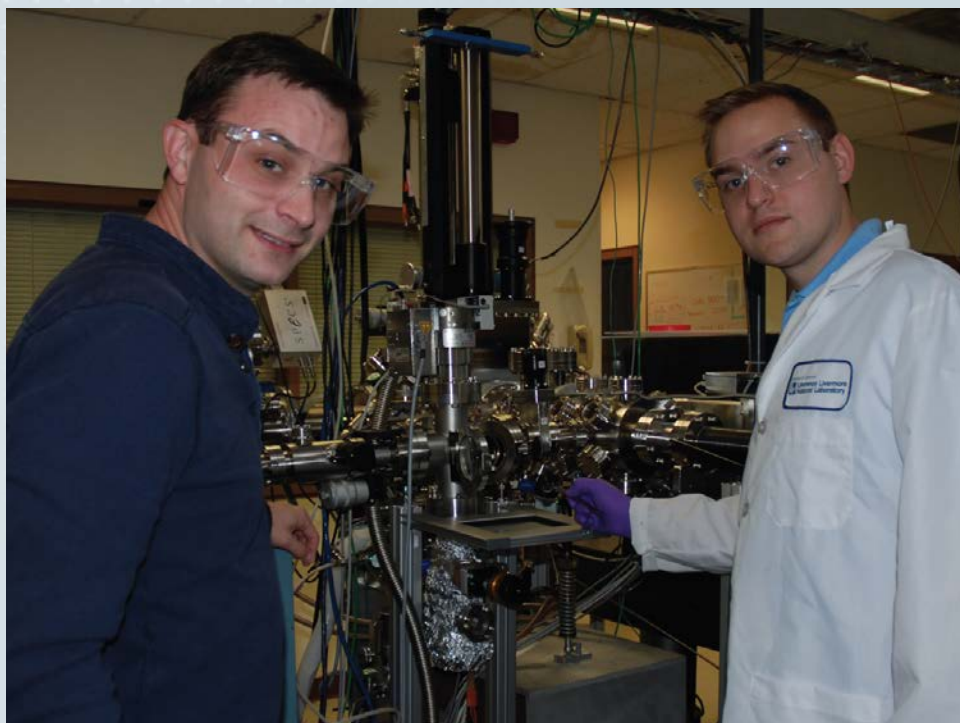
Research team members Jonathan Lee (left) and Michael Bagge-Hansen (right) prepare to test the vacuum integrity of a cell for in situ x-ray spectroscopy measurements of electrical energy storage materials.
