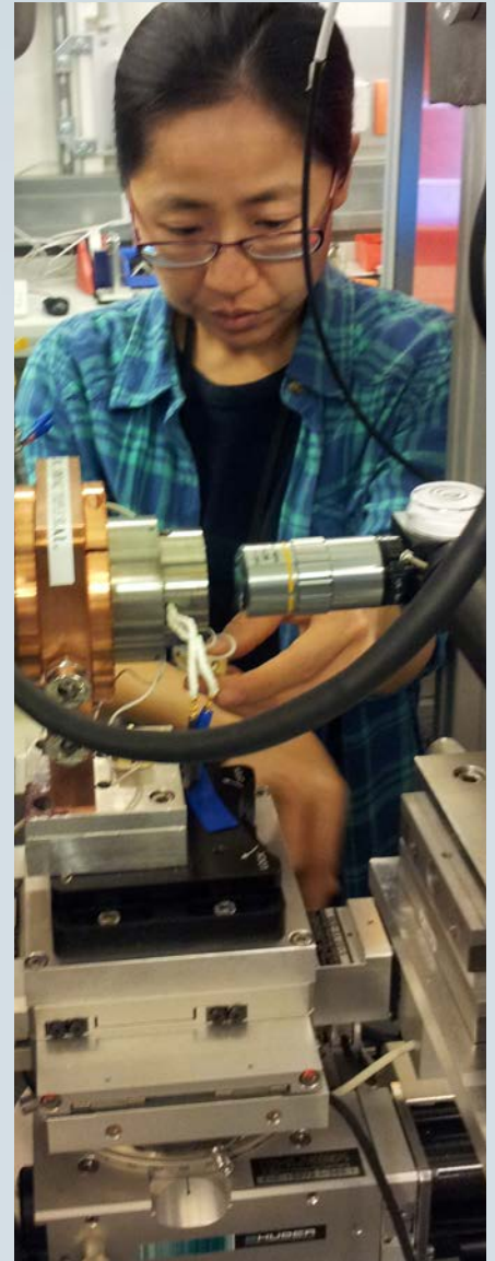
The Livermore dynamic diamond-anvil cell is used to study the influence of compression rate on the pressure-induced freezing, growth, and morphology of liquid metals. Here, researcher Jing-Yin Chen is setting up the anvil cell for operation at the extreme conditions beam line located at the Petra-III third-generation synchrotron x-ray source at DESY in Germany.
