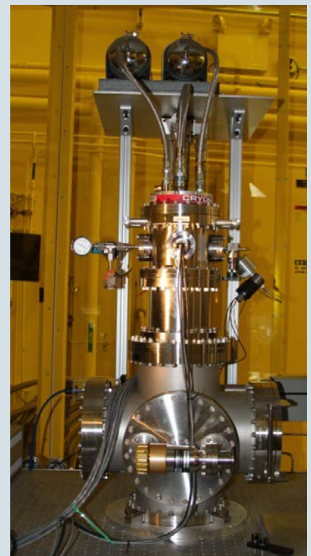
Cryostat used to measure depressed freezing temperature of hydrogen isotopes in ultralow-density foams used in laser fusion targets.
