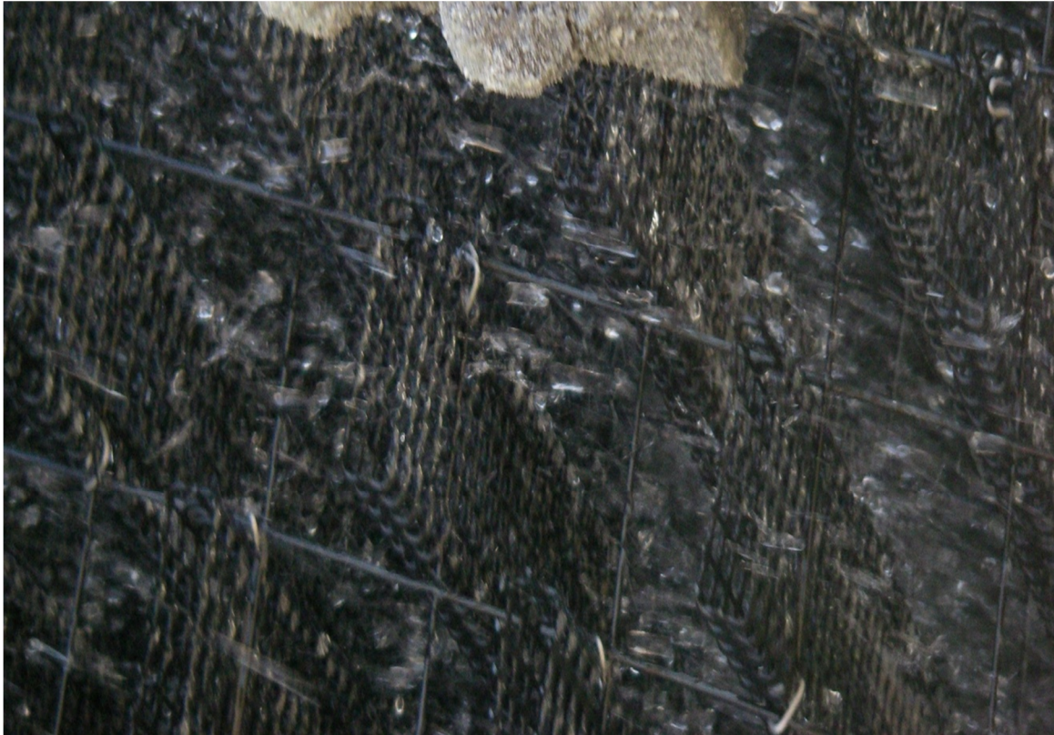
Figure 10. High efficiency PVC cooling tower fill from the field trial
