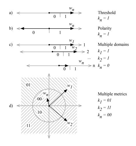
**Figure 2.** Previously demonstrated systems utilized a single metric converted directly to binary using threshold magnitude (a), signal polarity (b), or thresholds (c) at several frequencies. With with the measure of multiple uncorrelated metrics over multiple domains, a multidimensional constellation (d) can be utilized.
