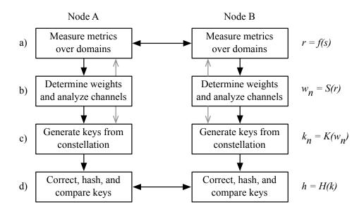
**Figure 1.** A generalized scheme for the creation of shared private keys through uncorrelated reciprocal channels in multiple domains. In (a) a signal, *s*, is transmitted across one or more channels in one or more domains and is received as a modulated signal, *r*. One or more domain-varying metrics,  $w_n$ , are measured (b) and converted to key symbols,  $k_n$ , using a key-generation function (c). The resulting key is error corrected and checked for agreement between nodes (d).
