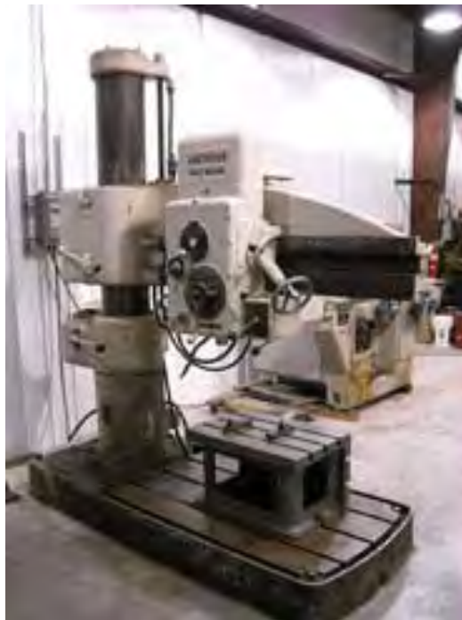
Figure 5 Radial Drill Press Like the One Used in This Experiment
