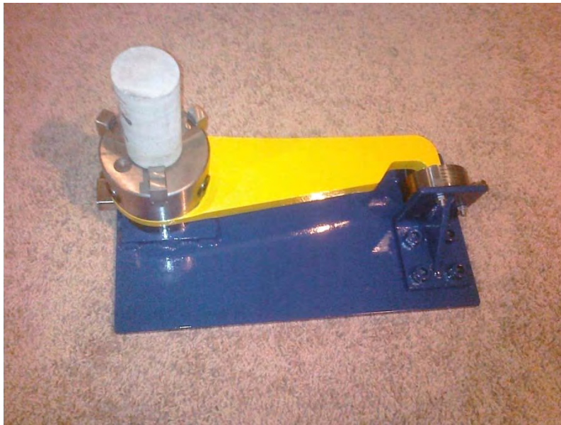
Figure 25 Rock Holding Fixture with Integrated WOB and Torque Load Cells
