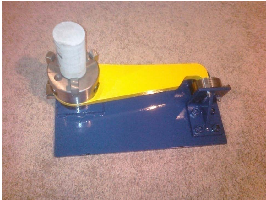
Figure 6 Rock Holding Fixture with Integrated WOB and Torque Load Cells
