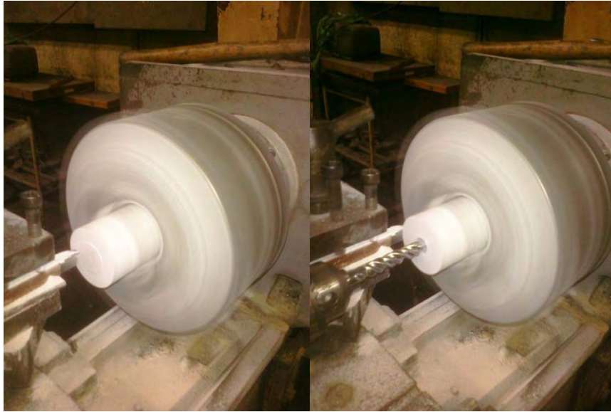
Figure 10 Left: Facing the End of the Sample. Right: Centering
