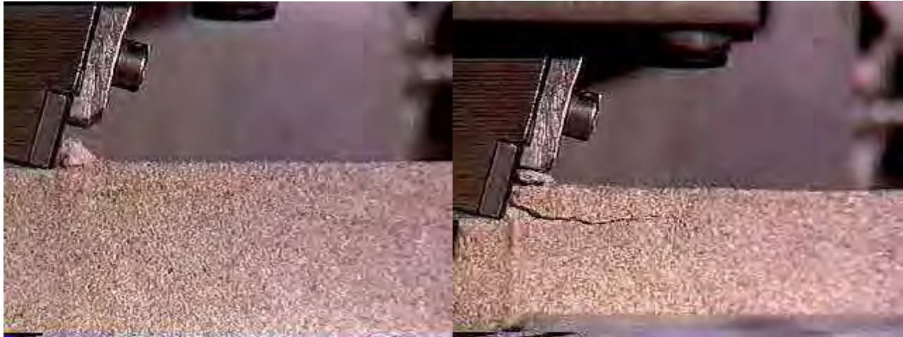
Figure 2 Comparison of Cutting Particle Size Between Small and Large Depth of Cut 34
