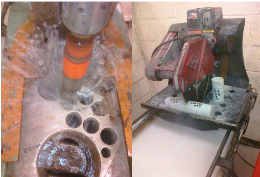
Figure 9 Rock Coring from Parent Slabs and Cutting Segments With Wet Saw
