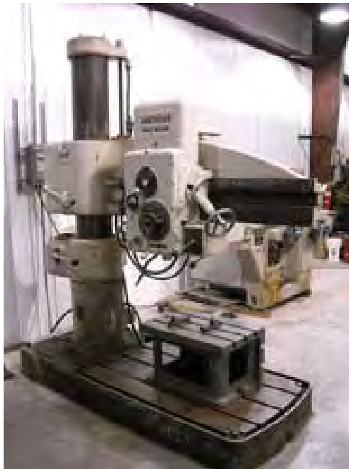
Figure 23 Radial Drill Press Like the One Used in This Experiment
