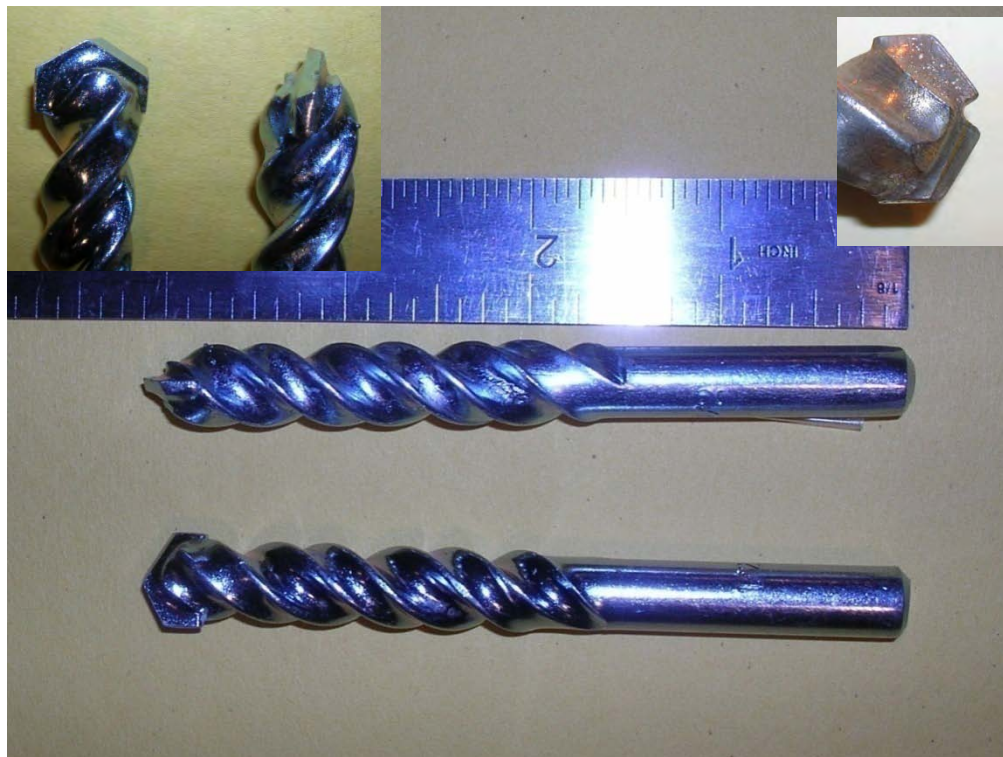
Figure 12 Drill Bits Used For All Experiments. Inset Left: Standard Tip. Inset Right: Two Wing Bit
