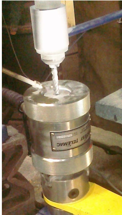
Figure 13 Hoek Cell Mounted in the Stiletto Apparatus. A Spacer Was Clamped in the Sample Holder, and the Hoek Cell Squeezed Both the Spacer and the Rock
