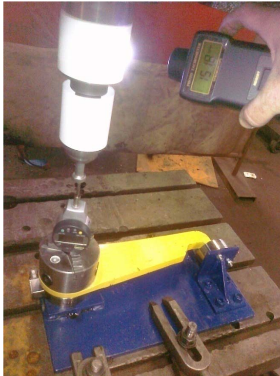
Figure 24 Calibrating the Penetration per Revolution of the Drill Press Used in Testing
