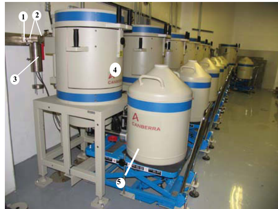
Fig. 2: The seven FPMS stations installed at the Advanced Test Reactor (ATR), which is located at the Idaho National Laboratory (INL).
