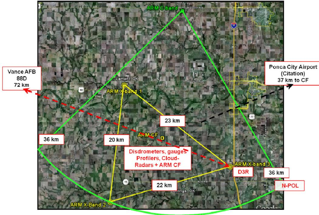
Figure 7. Nominal NPOL, D3R locations relative to MC3E radar network.
