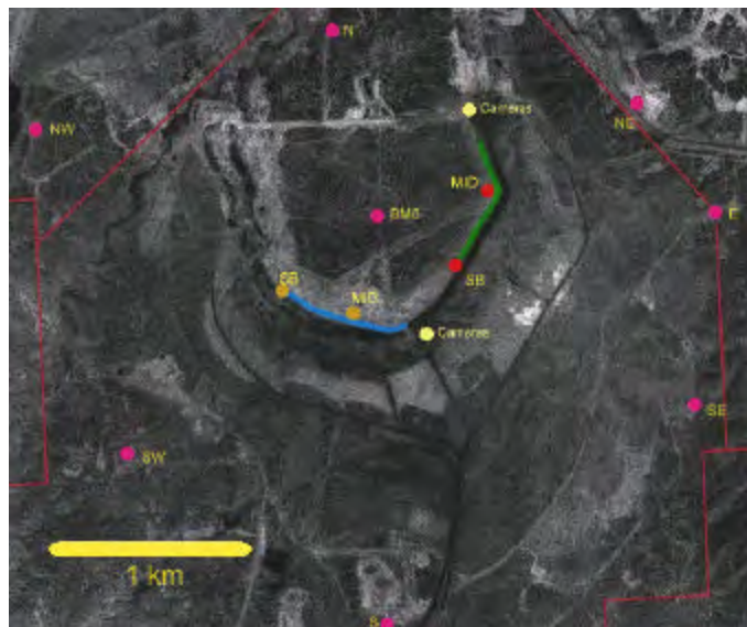
Figure 5. The locations of the seismic recording sites of the cast blast experiment for the 24 March 99 (Green) and 25 March 99 (Blue line) cast blasts. Each event was fired from station SB toward the station MID.
