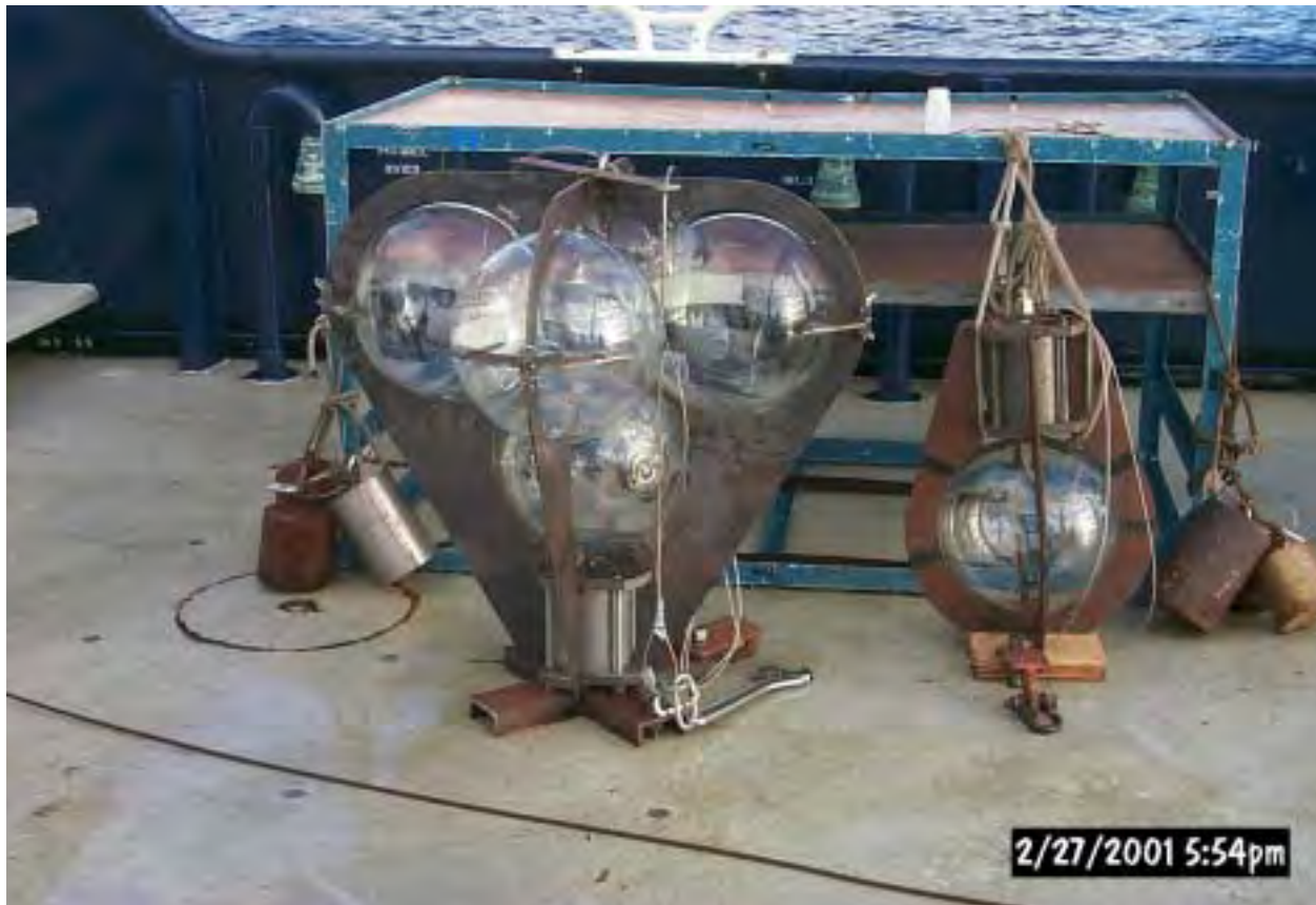
Figure 2. The prototype 5-sphere implosion system is shown next to the 1-sphere system. The smashing cylinder is the same for both.
