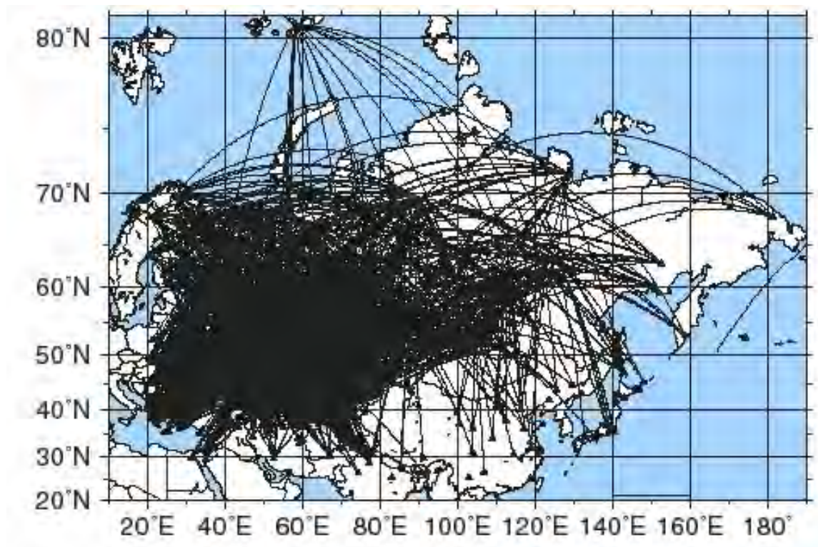
Figure 6. Great circle paths between the PNEs (stars) and stations (triangles) for which phase data are reported from 83 Soviet-era PNEs at standard and regional stations of the former Soviet Union and other stations in Eurasia, as collated by staff of the Institute of Dynamics of the Geosphere (Moscow). We have worked with several sources of information on station operations to resolve numerous questions of the station locations used in this dataset, which is a valuable resource for IMS station location calibration.
