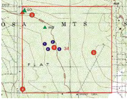
Figure 1. Map showing the geometry of the newly installed IMS infrasound station at Pinon Flat Observatory along with the IRIS 3-component broadband station. The eight microbarometer locations are plotted with circles and labeled L1-L4 (70 meter spaced filters) and H1-H4 (18 meter space filters), and the IRIS station is plotted with a triangle.
