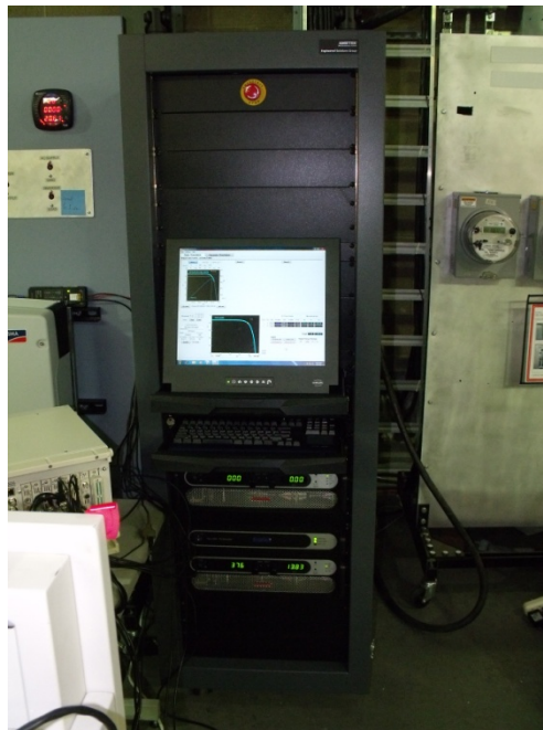
Figure 4.2. The TerraSAS PV solar simulator in EPRI's Knoxville lab.
