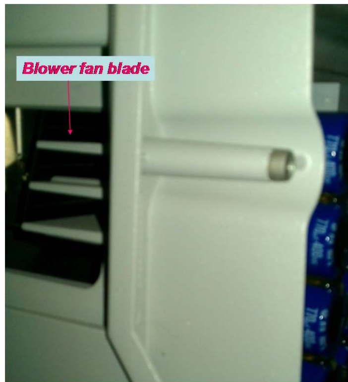
Figure 5.27. Photograph showing the blower fan section of the SunnyBoy 5000US 5-kW inverter.
