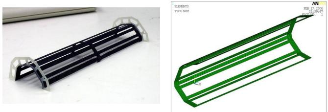
Carbon/Epoxy frame - cut away to save weight
