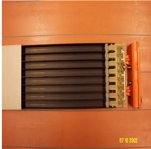
Figure 4.16: Picture of a LST installed in the barrel of BABAR .
