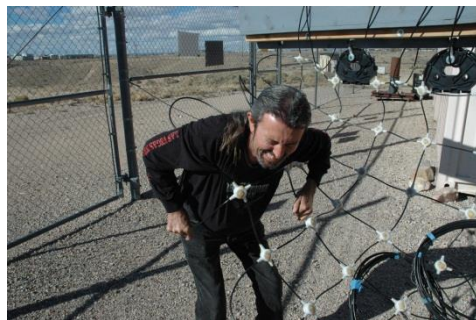
Figure 6. Stretching a Netting Sensor.
