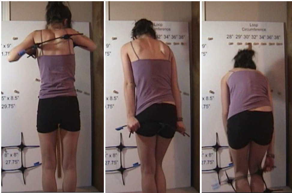
Figure A-3. Sequence Showing the Slipping of an 8.5-inch by 8.5-inch XSDS Aperture (29.75-inch circumference) from Head to Toe.
