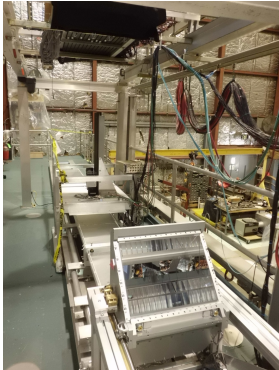
Figure 6: The photon camera and 5m-long bar box installed in the SLAC CRT. The picture shows the FBLOCK focal plane yet to be populated with detectors.
