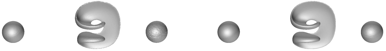
Figure 2: Reversal test of a 3D interface in deformation velocity field. The three plots in the left are computed in the 64^3 mesh, and the three right plots are in the mesh of 128^3 . For each set, from left to right are t = 0, 1.5, 3 respectively.
