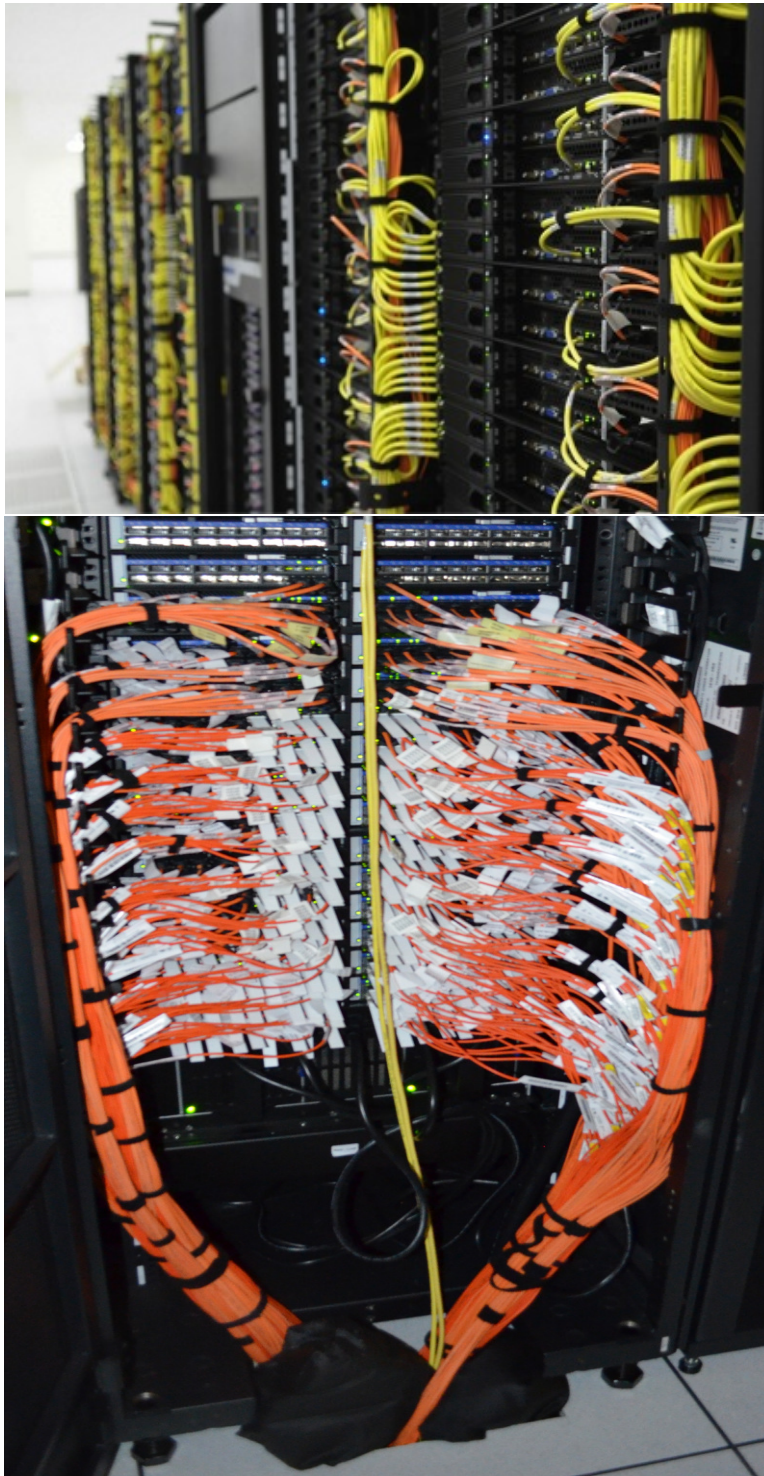
Figure 5.1: Photos of the Magellan System at Argonne. The top image shows the front of the compute cloud system as it is being installed. The bottom image shows the second IB rack after deployment of phase 2 hardware.
