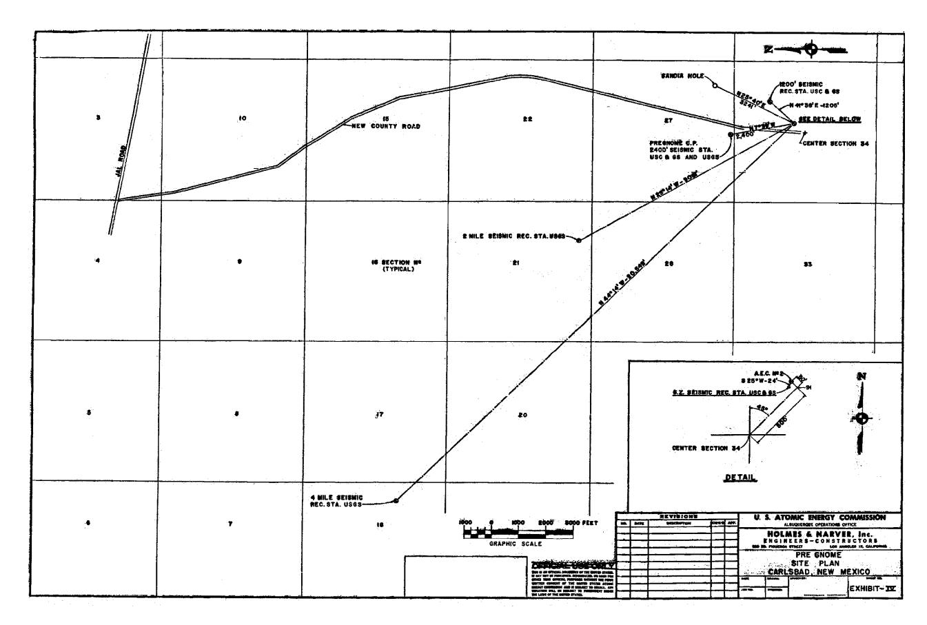
Figure 3.14-2. Location of seismic stations for Project Pre-Gnome (best available copy) (Holmes & Narver, Inc. [1959], no drawing number).
