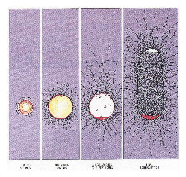
Figure 3.1-4. Proposed sequence of underground detonations for Project Bronco (Lekas et al 1967, Figure 3).
