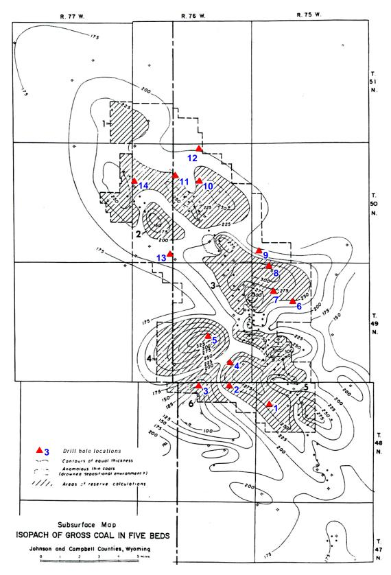
Figure 3.20-6. Locations of the 14 Project Thunderbird coal bed characterization drill holes completed between April and June, 1969 (adapted from Hicks and Woodward 1969, Fig. 2).
