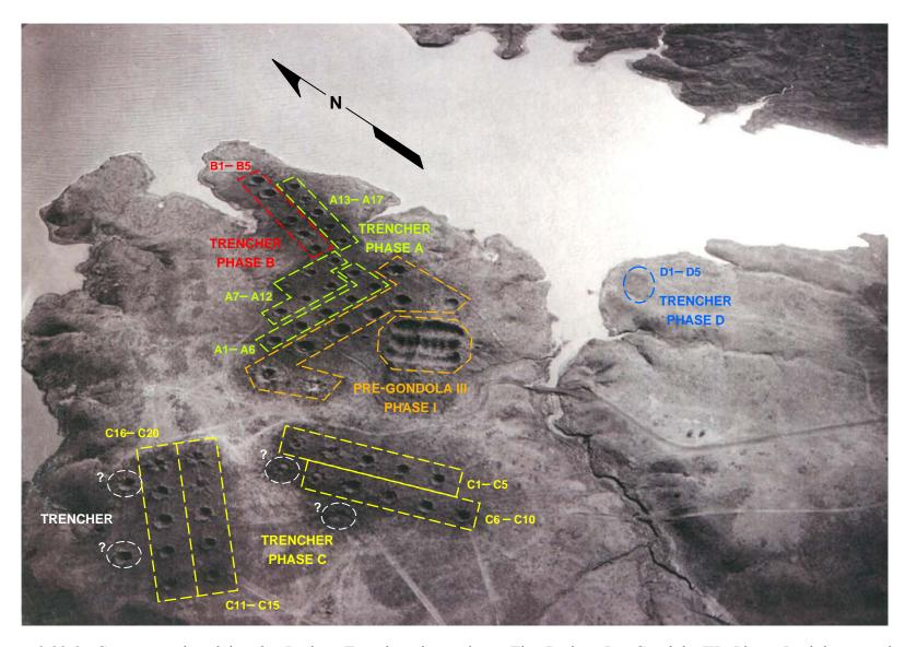
Figure 3.22-2. Craters produced by the Project Trencher detonations. The Project Pre-Gondola III, Phase I triple row charge experiment and eight calibration shots also appear on the aerial photo, c. Sept. 1969 (adapted from Lawrence Radiation Laboratory, U.S. Army Engineer Nuclear Cratering Group 1969).
