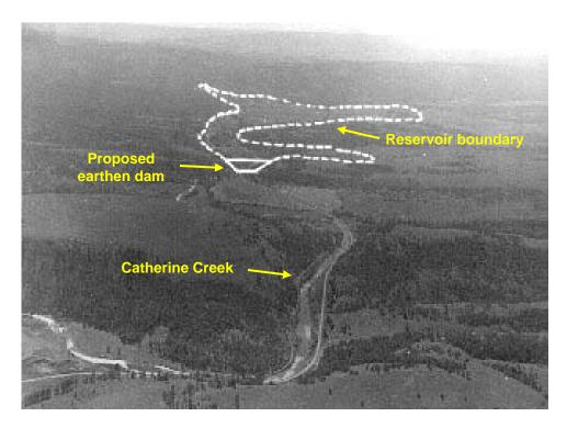
Figure 3.21-11. Conceptual drawing of the Catherine Creek dam site and reservoir, 1968 (adapted from U.S. Army Corps of Engineers, Walla Walla District website 2007, http://www.nww.usace.army.mil/dpn/f609a.htm, last accessed September 2008).
