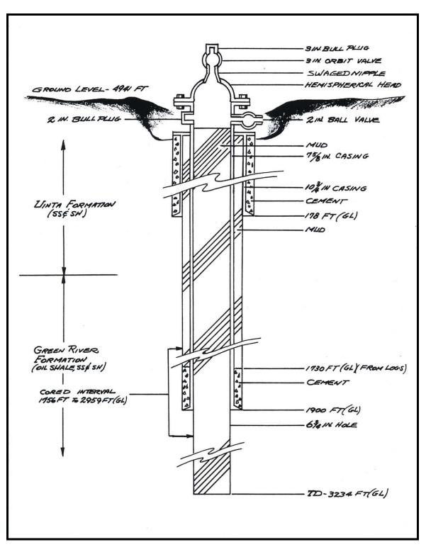
Figure 3.25-9. Schematic drawing of the WOSCO EX-1 drill hole (CER Geonuclear Corporation [1970], Figure 13).
