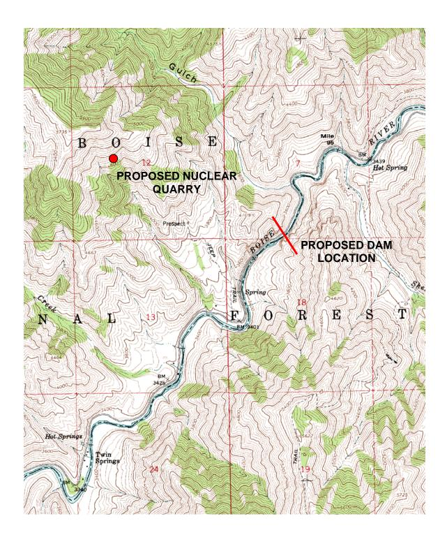
Figure 3.21-5. Both the Twin Springs, Idaho proposed dam and the proposed nuclear quarry are shown on this map (adapted from National Geographic Topographic Maps 2006).
