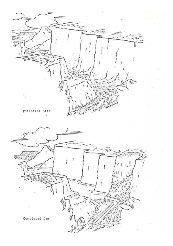
Figure 3.21-8. Schematic drawing for the Alternate #2 c oncept of a nuclear ejecta embankment dam (Kleist 1967, Figure 3).
