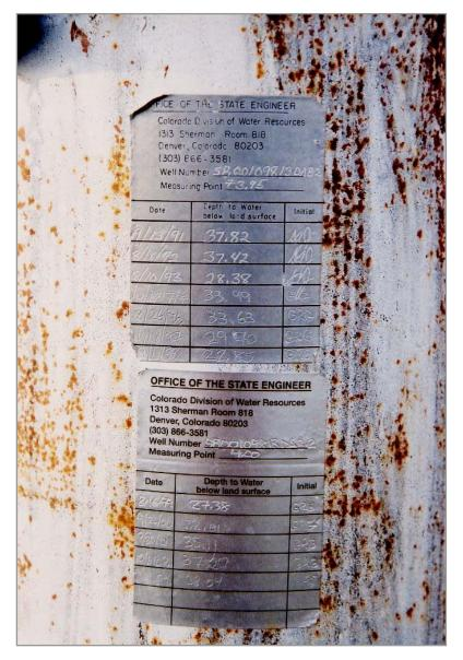
Figure 3.1-7. Office of the State Engineer, Colorado Division of Water Resources monitoring tags on Core Hole No. 1 (photo taken July 2005 on file at Desert Research Institute).
