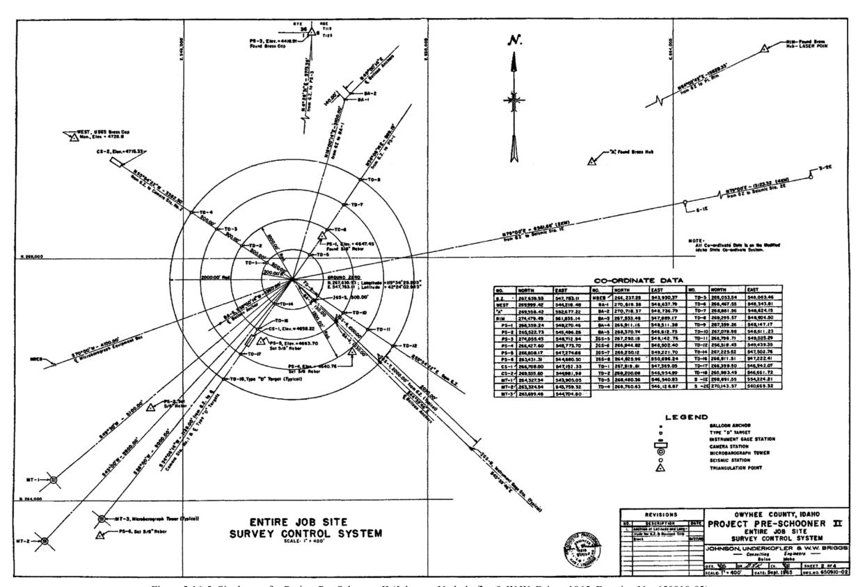
Figure 3.16-5. Site layout for Project Pre-Schooner II (Johnson, Underkofler & W.W. Briggs 1965, Drawing No. 650910-02).
