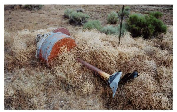
Figure 3.16-13. The surface motion targets are made of 8-inch diameter pipe with concrete-filled culvert collars. The targets were placed radially at varying distances from ground zero and recorded with motion picture cameras (photo taken July 2004 on file at Desert Research Institute).
