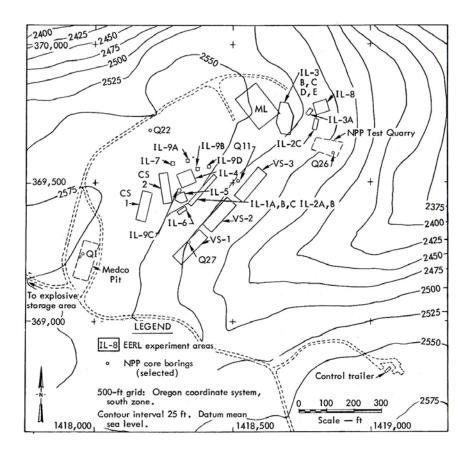
Figure 3.9-5. Site map of Project Lost Creek showing the location of experimental series of high explosive tests (McAneny 1975, Figure 2).
