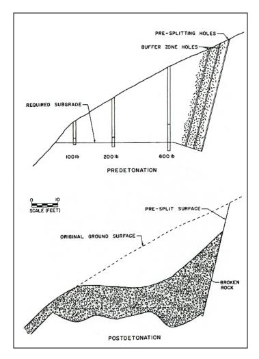
Figure 3.8-2. Schematic design for the Libby road cut experiment showing pre- and post-detonation cross sections (LaFrenz and Day 1972, Figure 8).
