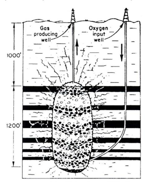
Figure 3.20-2. A nuclear detonation could be used to create the rubble chimney for in situ coal gasification (Wold and Woodward 1967, Fig. 2).
