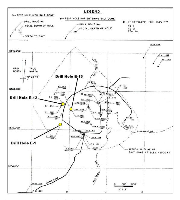
Figure 3.13-3. Map showing the location of drill holes E-1, E-12, and E-13 for Pre-Dribble at the Dribble site (the other drill holes are associated with Dribble) (adapted from Gardner and Downs 1971, Figure 6).
