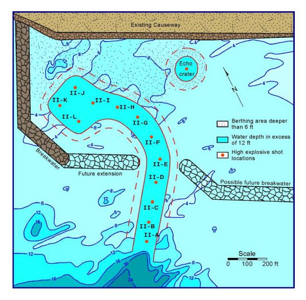
Figure 3.24-4. Plan view of the Phase II charge locations and the Phase I Echo calibration detonation (adapted from Day 1972, Figure 15).
