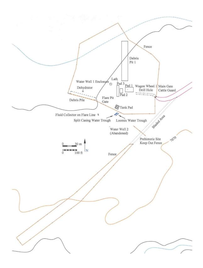
Figure 3.26-12. Plot plan of Project Wagon Wheel Site from FY 2003 field visit.
