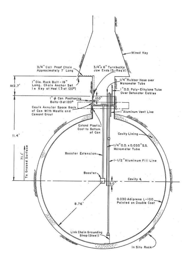
Figure 3.16-4. Schematic of the lower portion of the Pre-Schooner II emplacement hole, and explosive charge cavity (Hughes 1966, Figure 2.6).
