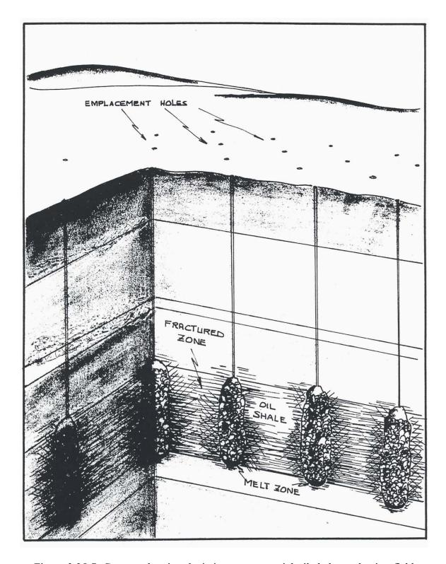
Figure 3.25-7. Concept drawing depicting a commercial oil shale production field with a multiple-shot array and a continuous zone of fractured rock (CER Geonuclear Corporation [1970], Figure 9).
