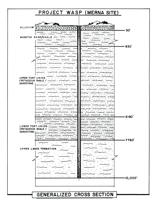
Figure 3.27-6. Generalized Cross Section the stratigraphy of Project WASP at the Merna Site (U.S. Atomic Energy Commission. Nevada Operations Office 1970, Figure 4).
