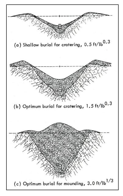
Figure 3.9-3. Illustration of the relationship between cratering and mounding as a function of depth of burst (McAneny 1975, Figure 3).
