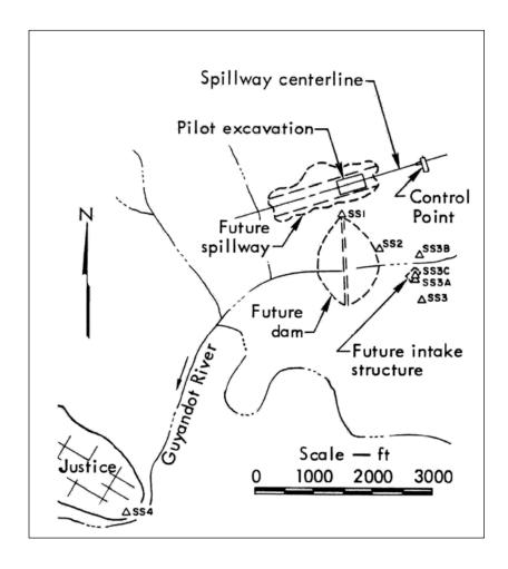
Figure 3.17-3. Location of the pilot excavation in relation to the proposed spillway and dam for R. D. Bailey (Bechtell 1975, Figure 69).
