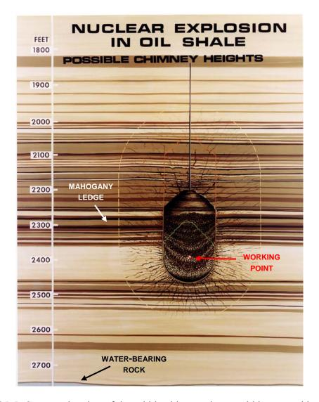
Figure 3.25-5. Concept drawing of the rubble chimney that would be created by a nuclear detonation in the barren zone just below the Mahogany Ledge oil shale deposit (adapted from Lawrence Livermore National Laboratory n.d., Negative No. GLC712-871A).
