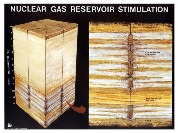
Figure 3.26-6. Schematic drawing of multi-shot models for nuclear gas reservoir stimulation experiments. The underground cross-section of the five 100-kt sequential shot Project Wagon Wheel experiment is shown on the right. The cutaway on the left depicts Wagon Wheel as part of a field of nuclear stimulated gas wells (Lawrence Livermore National Laboratory n.d.).
