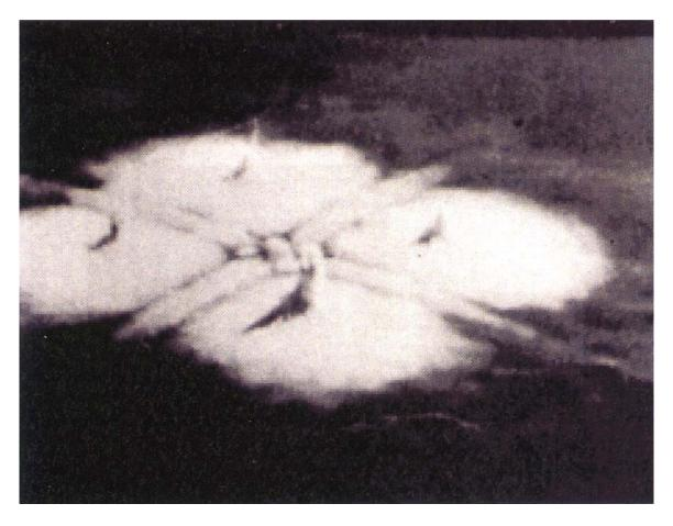
Figure 3.24-9. Detonations for the berthing basin showing the shock interaction and cavitation phenomenon of the four simultaneous blasts (Day 1972, Figure 45).
