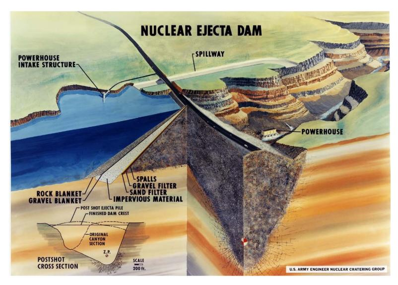
Figure 3.6-4. Nuclear ejecta dam concept (Lawrence Livermore National Laboratory n.d., Negative No. GLC-683-2152A).
