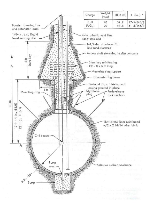
Figure 3.15-6. Cross section of chemical charge for Project Pre-Gondola (Kurtz and Redpath 1968, Figure 12).
