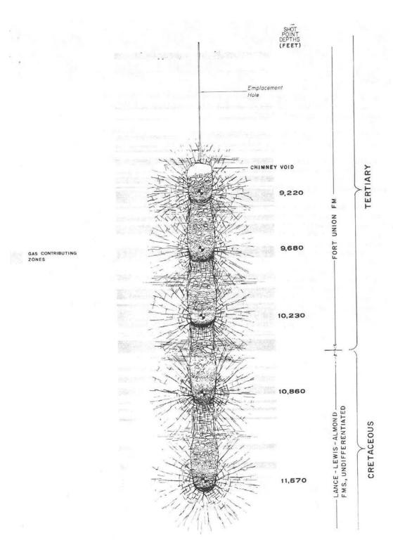
Figure 3.26-7. Project Wagon Wheel chimney region showing the proposed spacing of the explosive charges (U.S. Atomic Energy Commission 1972, Figure 2-3).
