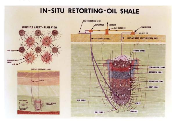
Figure 3.25- 6. Model for in situ retorting process using nuclear explosives to rubblize the oil shale deposit (Lawrence Livermore National Laboratory n.d., Negative No. GLC665-3753).
