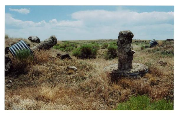
Figure 3.16-12. Target stands used in surface motion studies for the Pre-Schooner II detonation (photo taken July 2004 on file at Desert Research Institute).
