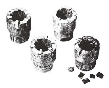
Figure 3.7-7. Expended drill bits from the Iki experiment. Top bit contains a cooled sample of molten lava (Rawson and Bennett 1961, Figures 6 and 7).
