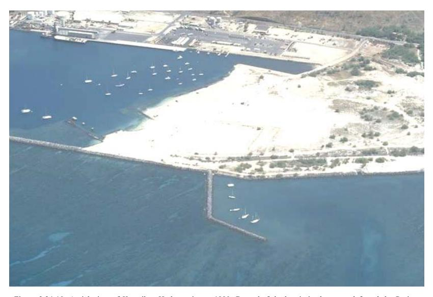
Figure 3.24-10. Aerial view of Kawaihae Harbor prior to 1990. Deep-draft harbor is in the upper left and the Project Tugboat light-draft harbor and breakwater are in the foreground. View is to the northeast (U.S. Army Corps of Engineers, Honolulu District).
