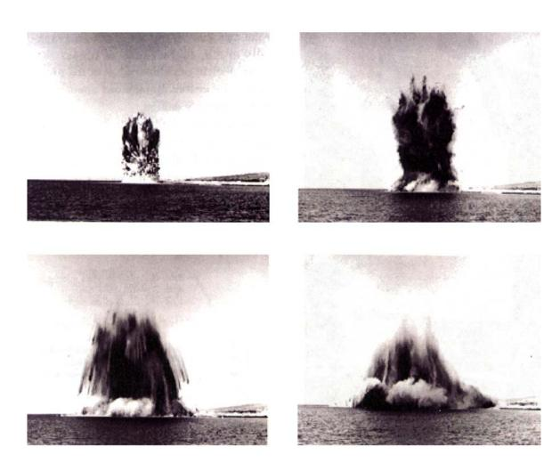
Figure 3.24-7. Sequential photos of Project Tugboat Phase I "Echo" calibration 10-ton detonation (Day 1972, Figure 36).
