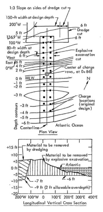
Figure 3.5-3. Illustration of the plan view and vertical cross section for the excavation and emplacement design of Drum Inlet (from Snell and Gillespie 1973, Figure 9).
