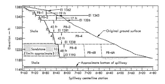
Figure 3.17-4. Profile of the pilot excavation showing major blast groups in relation to the five levels (Bechtell 1975, Figure 7).
