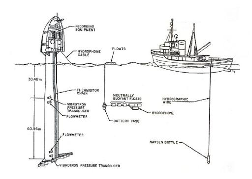
Figure 3.2-4. Hydrophone suspension system used for monitoring the CHASE V Detonation (Northrop 1968, Figure 2).
