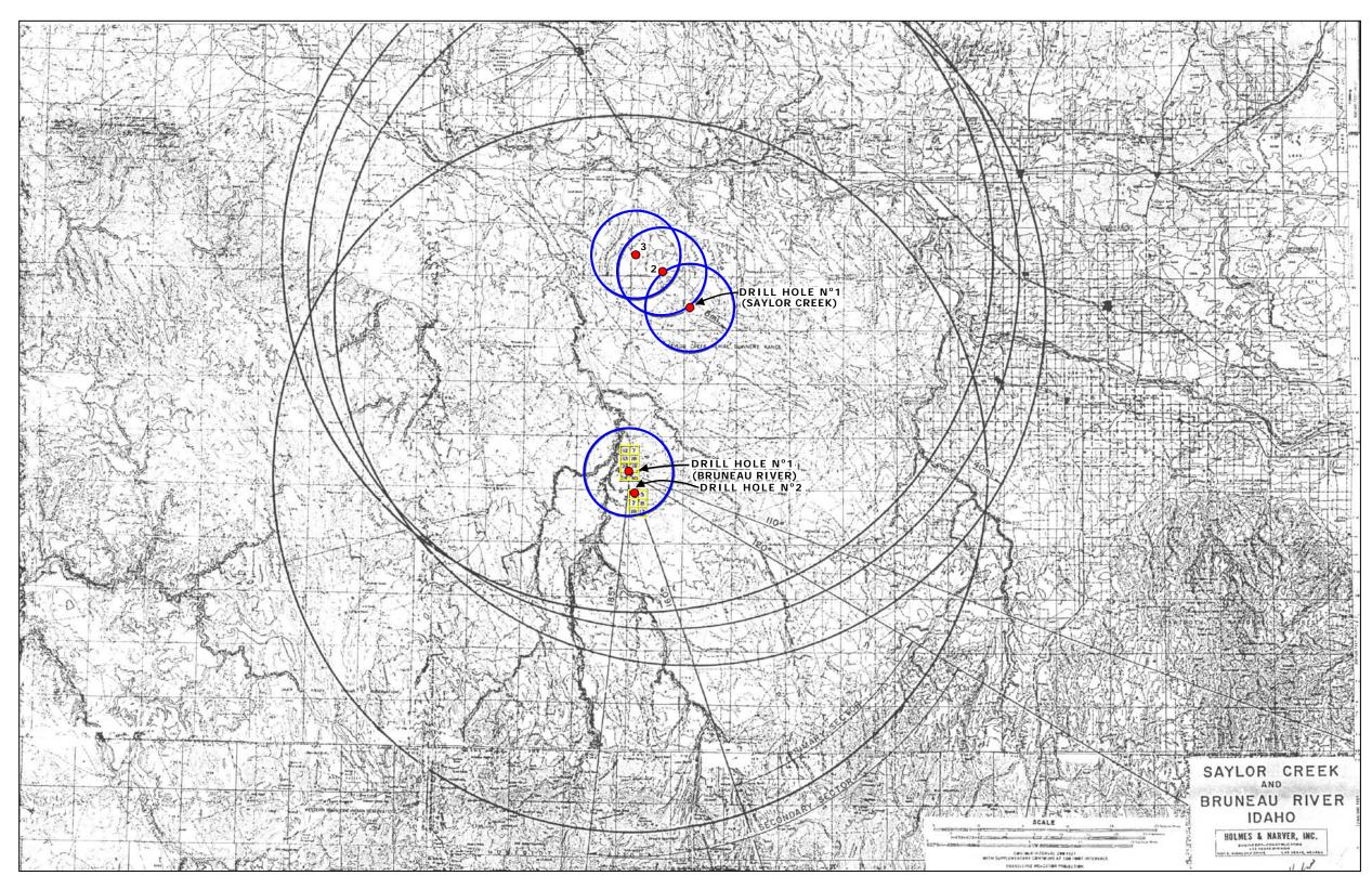
Figure 3.16-2. Some of site selection drill hole locations for the Pre-Schooner II experiment (adapted from Holmes & Narver, Inc. [1965b], no drawing number).
