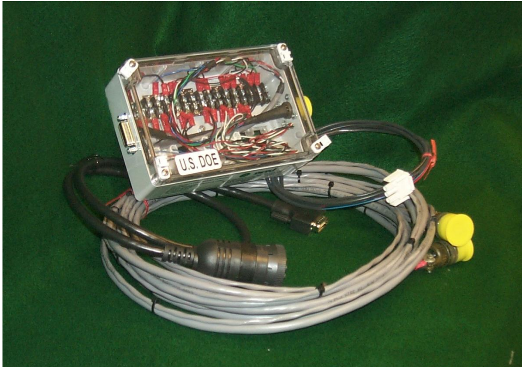
Figure 2. DASIB and associated cables.
