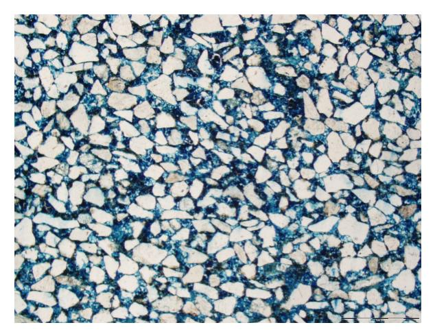
**Figure 90**. Griggs 107 1458' depth at red arrow in figure 12. This thin section is from 1458' depth indicated by red arrow in figure 70. This photomicrograph shows calcite cement stained dark navy blue indicating that the calcite is iron rich because the thin section was stained with a mixture of alizarine red containing potassium ferricyanide. The grains are fine-grained and angular. Porosity and permeability are minimal in intervals cemented by ferroan calcite.
