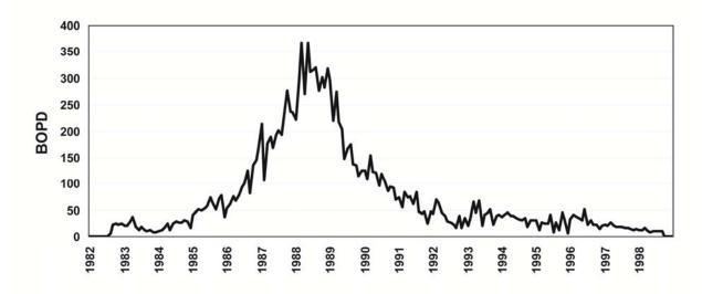
**Figure 4.** Graph showing increased production from the Robins 102-B Maraflood surfactant flood starting in 1982. The 25 acre Bridgeport B channel sandstone pilot project in the SE quarter of Section 5, T3N R12W achieved 34% SOR recovery (15% PV), 450 mbo. The flood was a scientific success but was not expanded. An oil price drop at this time apparently did not offset the cost of polymer and surfactant.
