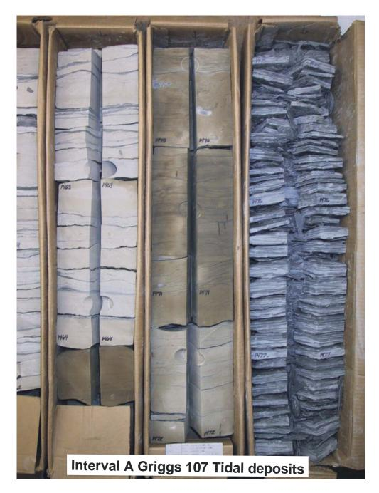
**Figure 69**. Core from Plains Illinois Griggs 107 well Sec. 32-T4N-R12W. Contact between oil stained reservoir quality sandstone with high core measured porosity and permeability values and interbedded, flaser bedded siltstone and shale permeability barrier.
