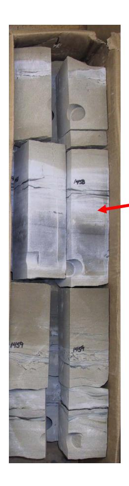
**Figure 70.** Calcite cemented sandstone indicated at red arrow, limited to a few inches to a foot thick, compartmentalizes the sandstones and is observed in all Cypress core from the pilot area.
