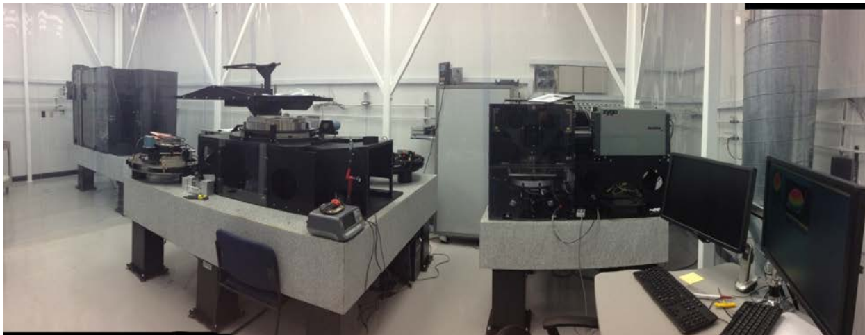
Figure 8. MET5 optical tests (left to right): POB transmitted wavefront test, M2 and M1 mirror surface figure tests.
