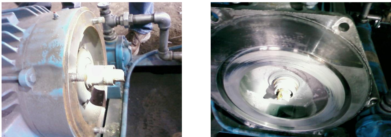
Figure 20. Pictures of the first vacuum pump motor installed in the Cholla membrane unit, showing the remaining shaft stub after the shaft was dissolved by the permeate gas.
