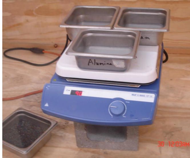
Figure 11: Process of water evaporation on a hot plate at 90°C
