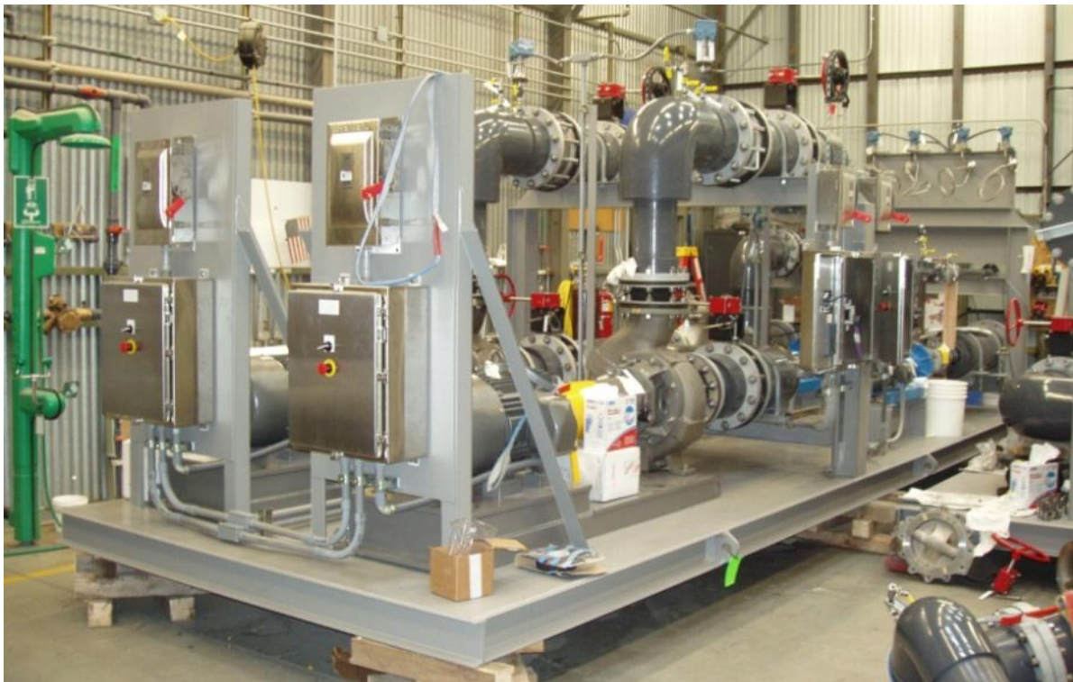
Figure 13 - 2W P&T Fluidized Bed Reactor Pump
