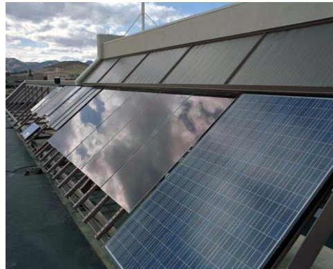
Figure 2 Performance Energy Rating Testbed (PERT) at NREL. Photo credit: Warren Gretz, NREL PIX 03877.
