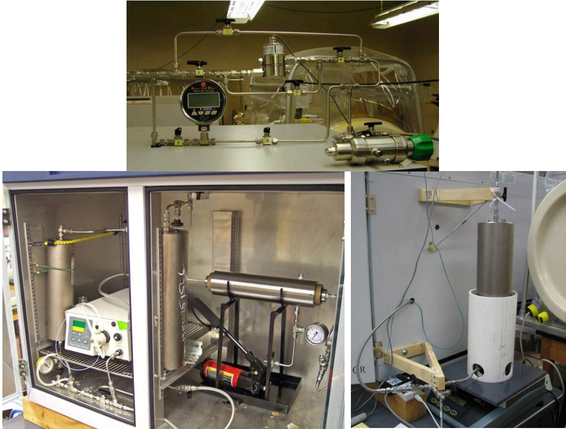
Figure 4. High Pressure Biofilm and supercritical CO 2 testing apparatus: TOP- Series of valves and gauges that allow differential pressure setup BOTTOM LEFT - Accumulator for nutrient storage, supercritical CO 2 storage accumulator (far left), Hassler-type core holder with Berea sandstone core, (all housed inside an incubator for temp. control) BOTTOM RIGHT - Accumulator and sample port used to collect effluent samples.
