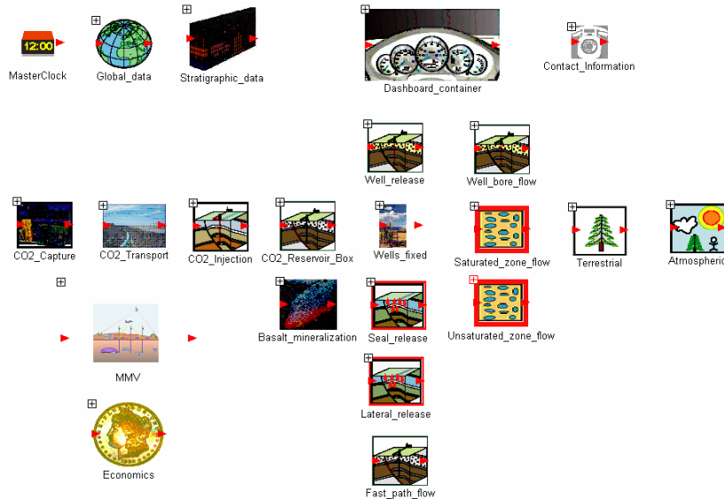
Figure 55. First version of the GoldSim systems model, CO 2 -PENS, developed at LANL
