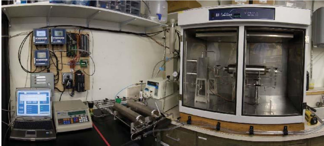
Figure 3. Version 3 of the flow-through reactor system. (A) Photograph and (B) Schematic diagram showing flow-through reactor used in experiments.
