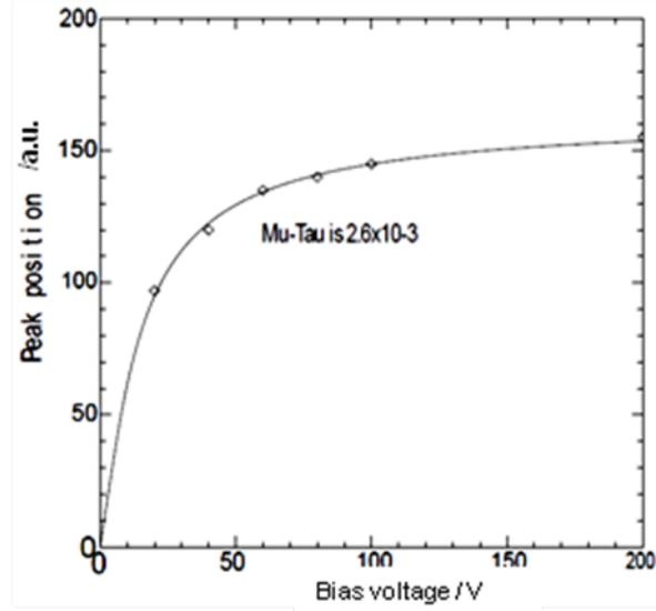
Fig. 6 Plot of charge collection as a function of applied bias voltage in the crystal from the stable growth region
