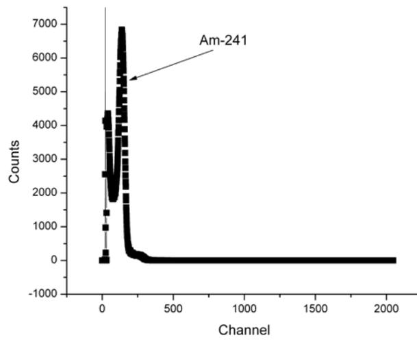
Fig. 5 Energy spectrum of the CMT crystal from the stable growth region (A sealed source Am-241 was used in the measurement).
