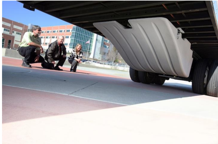
Figure 4.2. Trailers equipped with BMI Corp. SmartTruck UnderTray components can achieve a 7-12% percent improvement in fuel mileage. Representatives were on hand at ORNL on March 1, 2011 to display the components.
