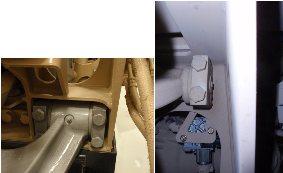
Figure XIII-1 Pillow Blocks Mounting the Control Arm to the Frame
