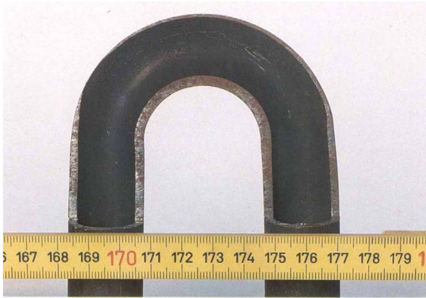
Figure 19. Erosion/Erosion Corrosion on a pipe [39]. Note that this is not piping from the SRS transfer line system.
