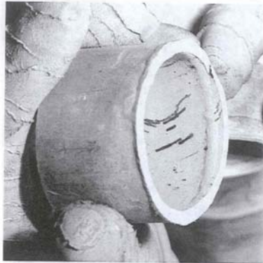
Section of failed catheter, with dye penetrant illustrating cracks at the leak site.
