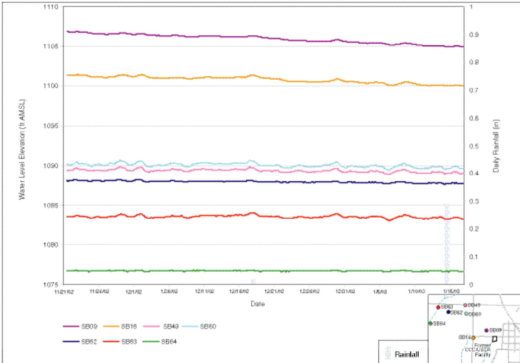
FIGURE 4.14 Hydrographs from the Everest water level monitoring network, with daily precipitation recorded at Horton, Kansas, from November 21, 2002, to January 17, 2003. (Complete data are in Appendix D, Table D.5, of the present report.)
