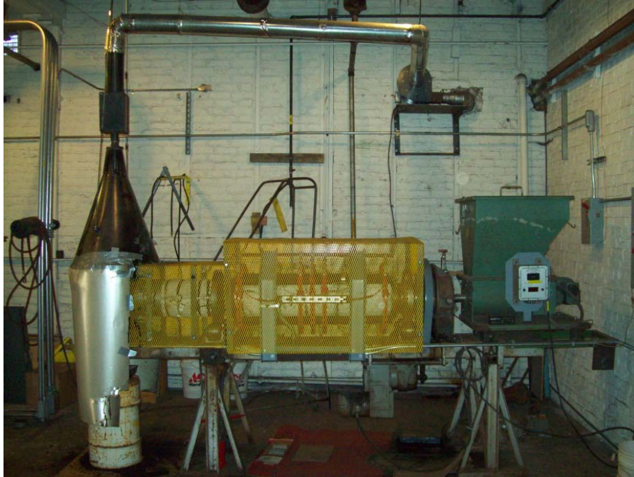
Figure 6: Completed Rotary Calciner Torrefier at NRRI
