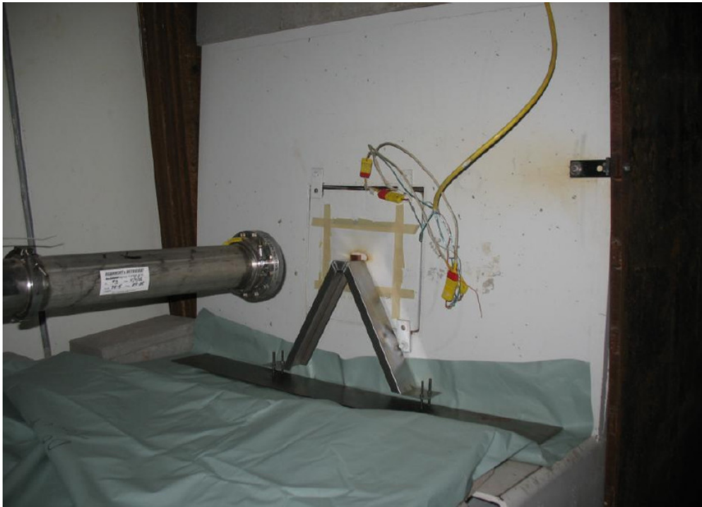
Figure 6: Target holder mounted in front to the 8GeV beam dump of the booster
