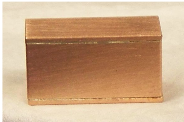
Figure 5: Target assembly – copper housing with thorium target inside
