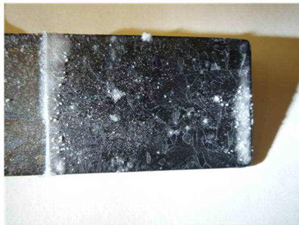
Figure 5. Photograph of salt on uncoated mild steel surface
