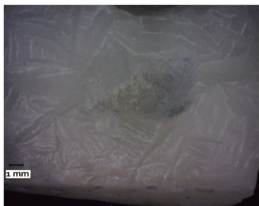
Fig 4 Ingot as cast pattern for NaNO 3 with 98% purity
