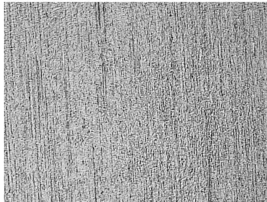
Figure 29. Electropolishing in 60% Sulfuric acid and 20% Phosphoric acid for 30 minutes. 100X
