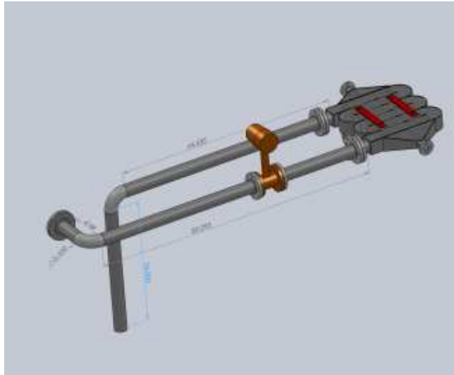
Heat exchanger overview, including inlet and outlet pipe runs and flow meter.
