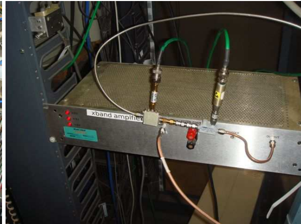
Figure 36: Photograph of the phase mixer with LO signal from station 0, and RF signal from station 2.
