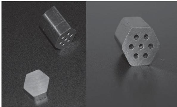
Figure 4. Tungsten nuclear thermal rocket fuel elements loaded with  $\text{CeO}_2$  (40% vol.), which acts as the  $\text{UO}_2$  simulant. The samples were fabricated using the Spark Plasma Sintering furnace.
