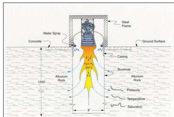
Figure 6. Schematic of the SAFE testing concept.
