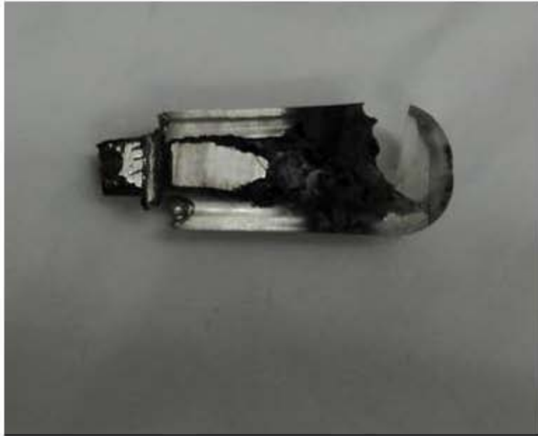
c) The damaged Inconel 690 coupon cross sectioned after mounting in epoxy.
