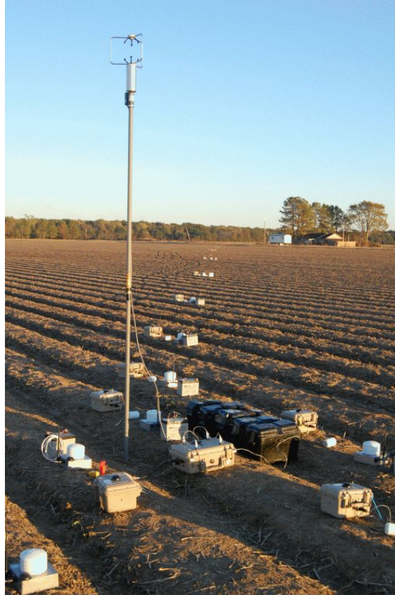
Fig. 3.23. View of the test site looking South-East from the array center. The sonic anemometer shown is positioned 124 inches above the ground.
