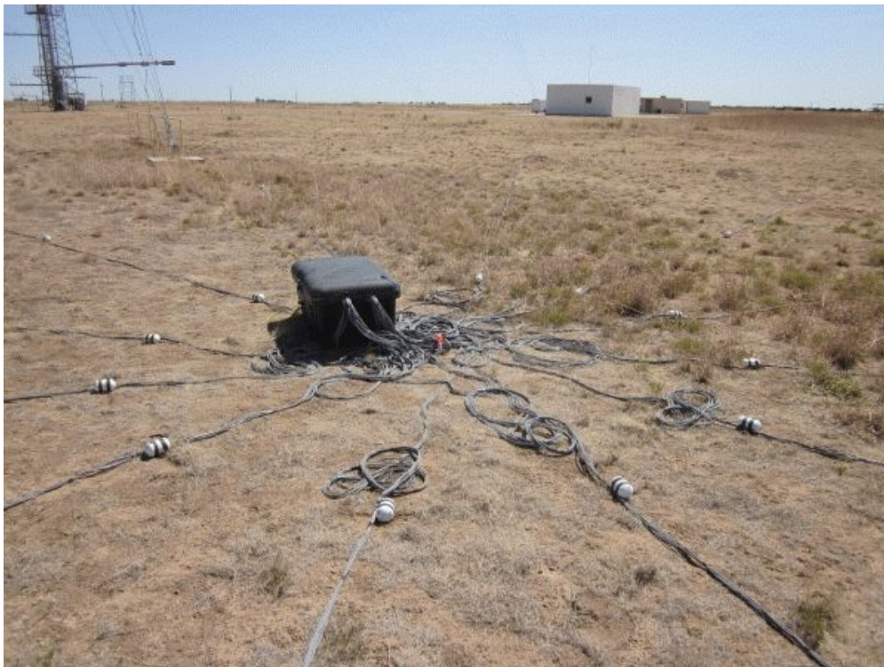
Fig. 3.33. Small aperture array setup for the Lubbock, TX, experiment.
