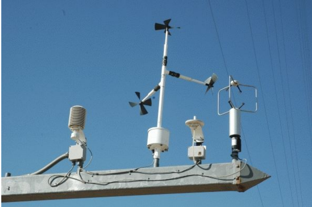
Fig. 3.32. The meteorological tower at the Reese Technology Center includes measurements at 10 stations. This photo shows the equipment at each station which include a sonic anemometer, propeller anemometer, temperature sensor, and humidity sensor. Three of the stations include a barometric pressure measurement.
