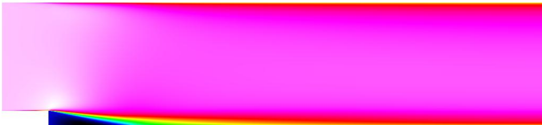
Figure 2: Mean streamwise velocity, U in the mid-span plane of the wind tunnel.
