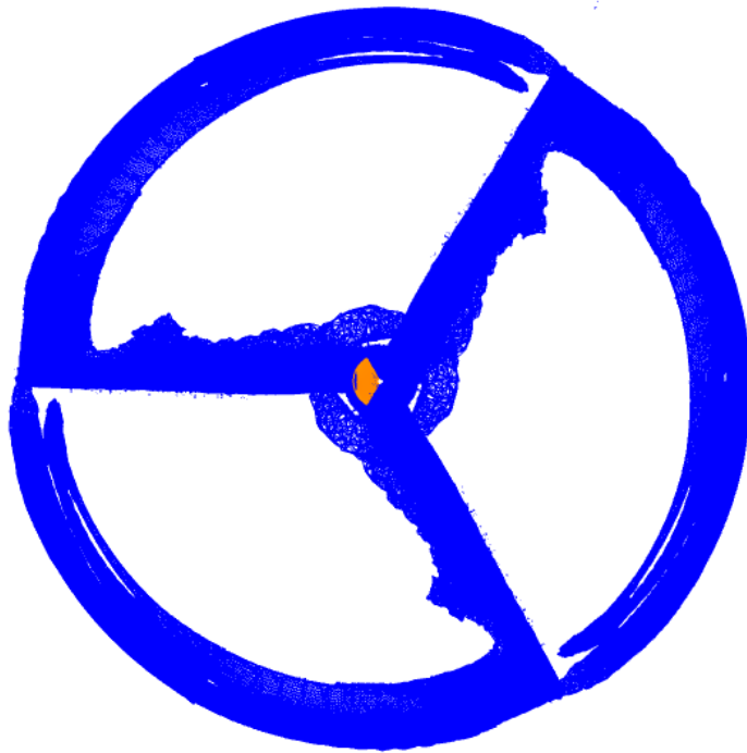
Figure 29: Iso-surface of Vorticity showing Tip Vortex and vorticity production around the blades.
