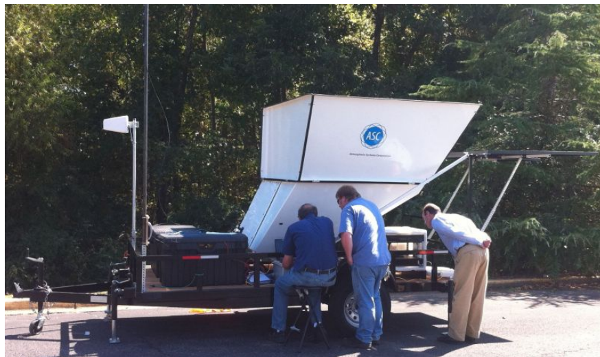
Fig. 2.3. The Atmospheric Systems Corporation multi-beam Doppler SODAR used in the present investigation.
