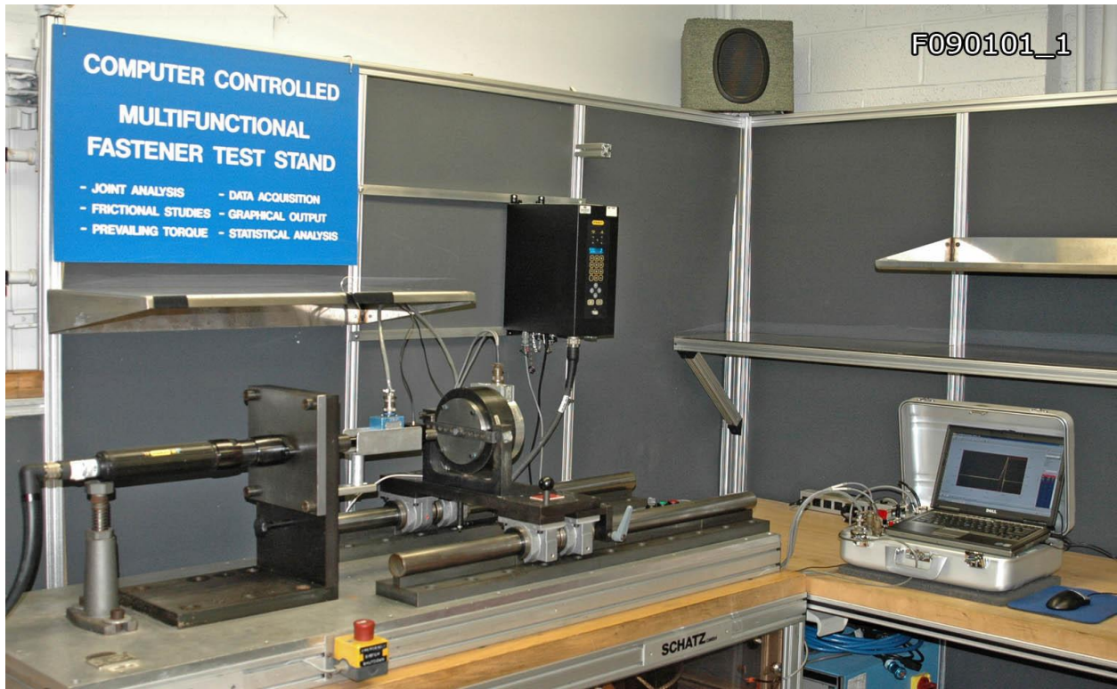
Fig. 7.7 Ford Fastener Laboratory Clamp Load Test Cell
