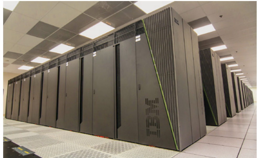
After a yearlong integration period, Sequoia's 96 racks, 1.6 million cores, 1.6 petabytes of memory, and 20 quadrillion floating-point operations per second are yielding impressive scientific results. Photo by Ross Gaunt.
