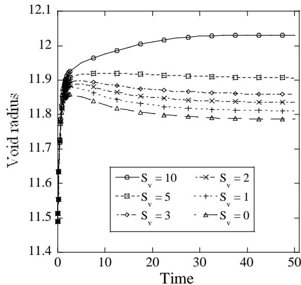
**Figure 1.** Void radius as a function of time for different initial vacancy supersaturation levels.
