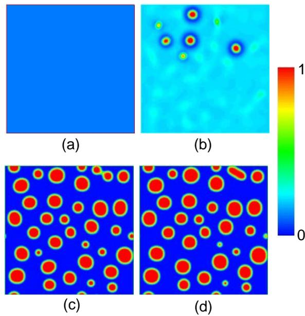
**Figure 3.** Display of the vacancy field illustrating the concurrent void nucleation and growth in a supersaturated system under the effect of stochastic vacancy generation: (a) initial system, (b), (c) and (d) evolution snapshots.
