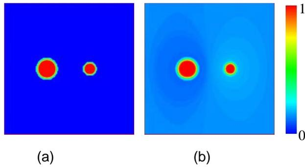
**Figure 2.** Evolution of concentration field around two interacting voids: (a) initial field and (b) a snapshot of the system at a later time. The concentration field is depressed around the larger void due to vacancy absorption, and it is higher than the remote background values closer to the small void due to vacancy emission.
