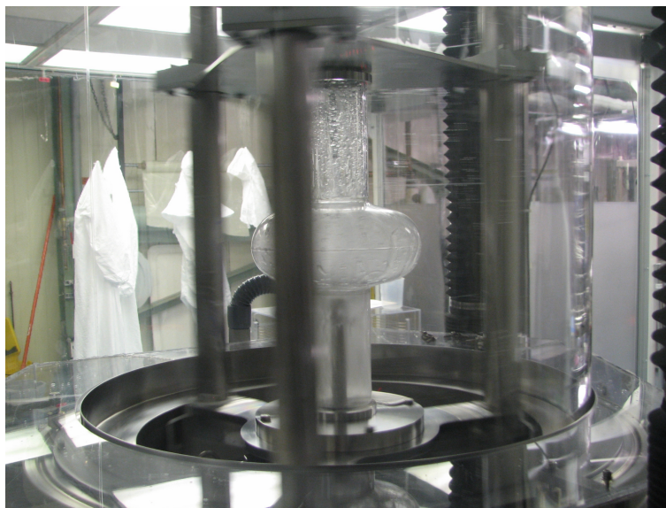
Figure 9 High pressure rinse of clear plastic model cavity
