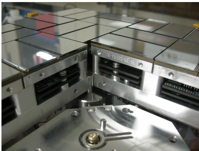
Fig. 3. The camera in construction, showing three of four quadrants.
