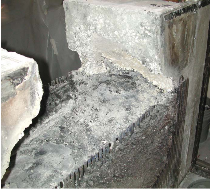
Figure 4-35. Solidified Corium and Concrete Sidewalls (View From Southeast).
