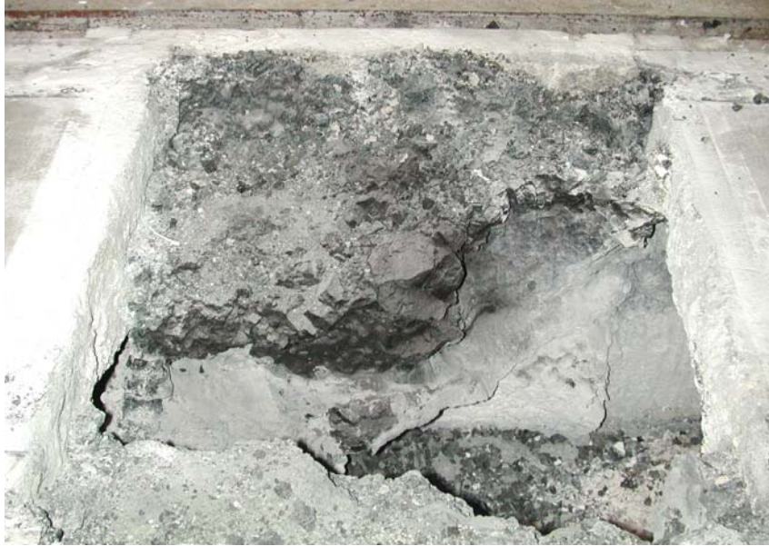
Figure 4-33. Crust Mantle Adhering to East Sidewall (after removal of bridge crust).
