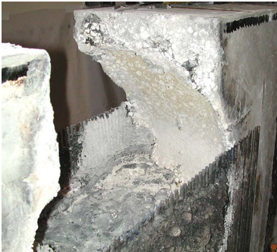
Figure 4-36. Solidified Corium and Concrete Sidewalls (View From Northwest).
