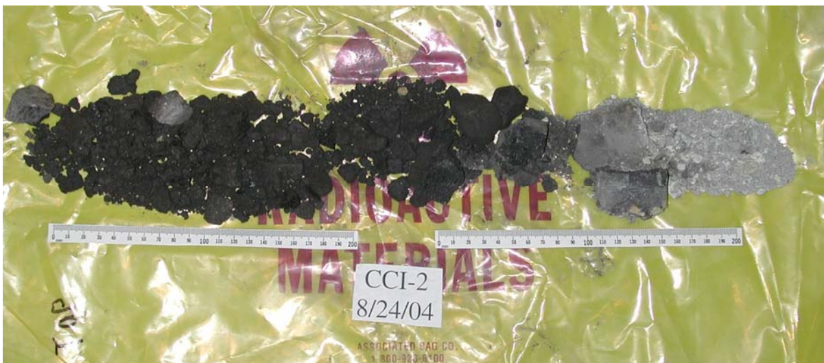
Figure 4-38. Core Sample Remnants (Core-concrete interface is to the right).
