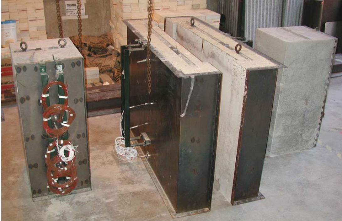
Figure 2-7. Photograph Showing Lower Section Sidewall Components After Fabrication.
