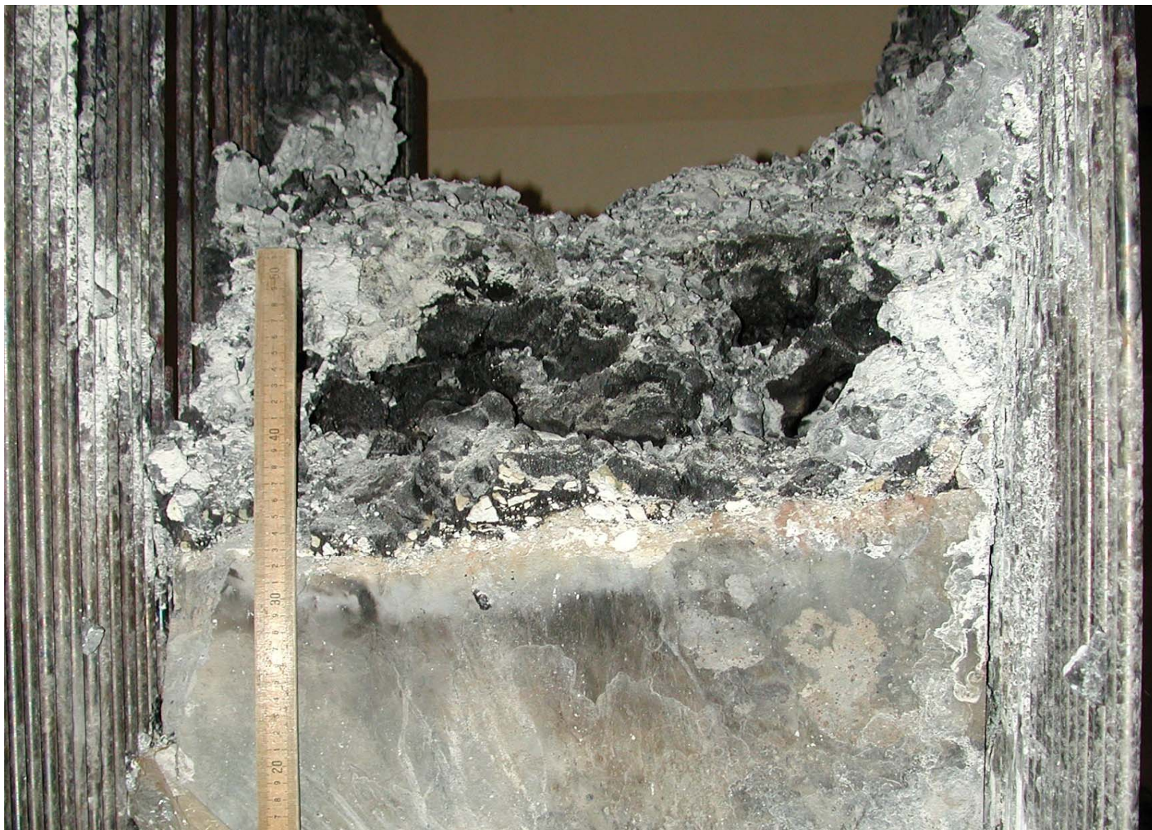
Figure 4-39. View of Solidified Corium Remaining Over the Basemat.
